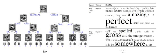
**Figure 8.** Examples of rule-based explanations generated by XAI methods for neural networks and visualised as (**a**) decision trees (Decision Tree Extraction [86]), or (**b**) by showing the most relevant input (Word Importance Scores [94]).
