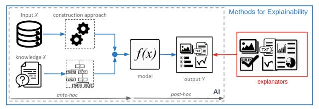
Figure 1. Diagrammatic view of how an explainable artificial intelligence (XAI) solution is typically constructed.
