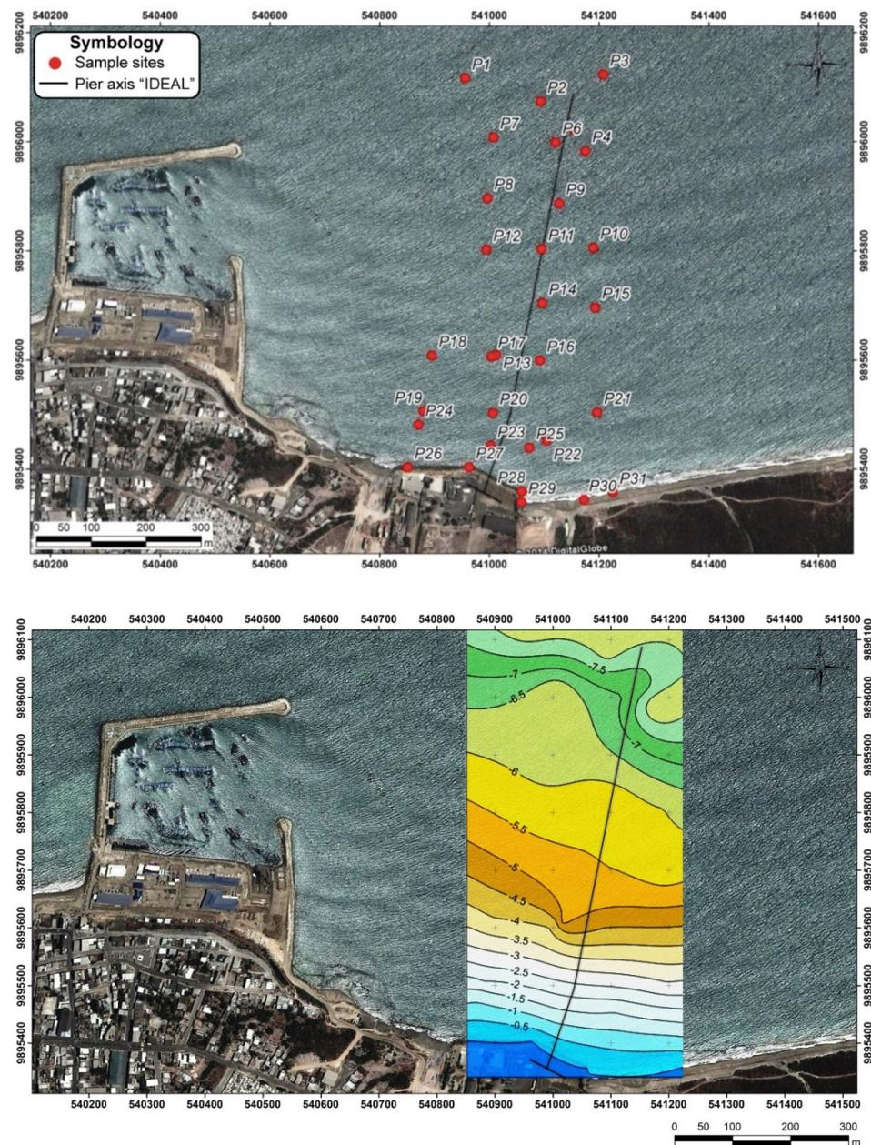
**Figure 5.** Bathymetry map in the sector of the Ideal dock and the Jaramijó river. Note, in the western sector, the artisanal fishing pier of Jaramijó. The depth isobaths are expressed in meters.
