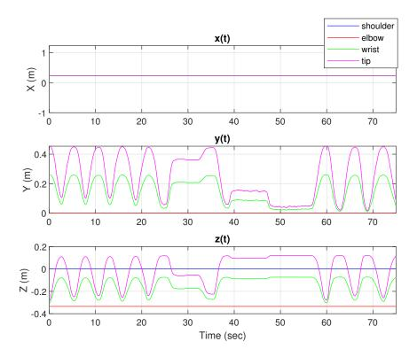
**Figure 5.** Joints trajectories coordinates in *x*, *y*, *z* axes for elbow flexion-extension exercise—Custom-made sensor node.
