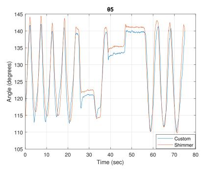
**Figure 4.** Elbow rotation angle  $\theta_5$ —Pronation-Supination DoF.
