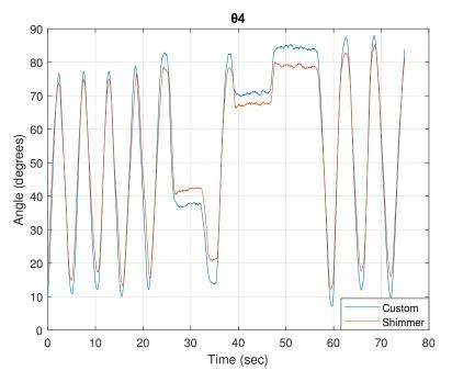
**Figure 3.** Elbow rotation angle  $\theta_4$ —Flexion-Extension DoF.
