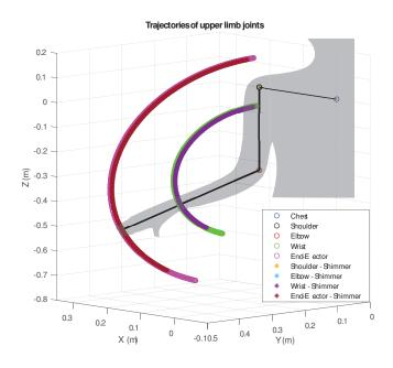
**Figure 6.** Wrist and hand trajectories during elbow joint flexion-extension exercise – Comparison with Shimmer3 sensor nodes.
