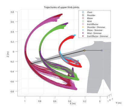
**Figure 11.** Elbow, wrist and hand trajectories during shoulder joint abduction-adduction exercise – Comparison with Shimmer3 sensor nodes.
