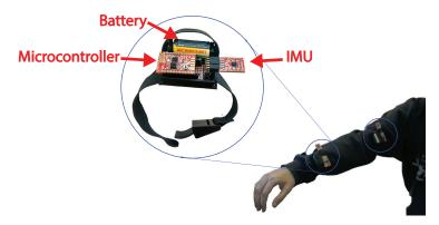
Figure 2. The wearable motion sensors.
