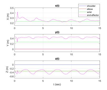
**Figure 14.** Joints trajectories coordinates in *x*, *y*, *z* axes for wrist flexion-extension exercise—Custom-made sensor node.
