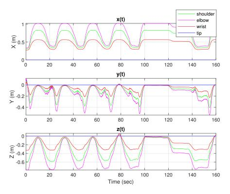
**Figure 10.** Joints trajectories coordinates in *x*, *y*, *z* axes for shoulder abduction-adduction exercise—Custom-made sensor node.
