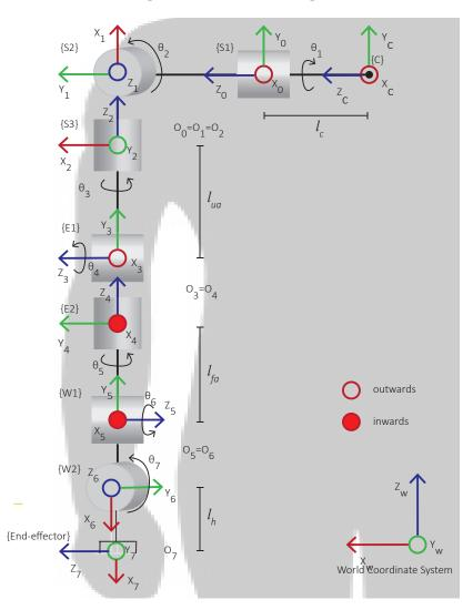
for the wrist joint DoFs, namely flexion-extension and deviation. The end-effector position and orientation correspond to the ones of the tip of the hand.
