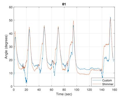
**Figure 7.** Shoulder rotation angle  $\theta_1$ —Flexion-Extension DoF.
