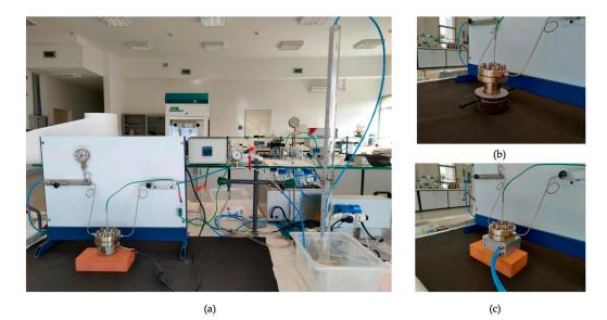
**Figure 2.** HTC apparatus: (**a**) HTC system during heating phase; (**b**) HTC reactor cooled down through a massive stainless steel disc at -10 °C; (**c**) HTC reactor cooled down through a stainless steel radiator with flowing tap water.
