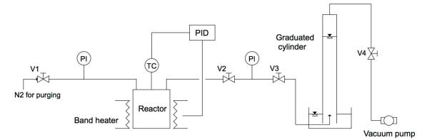
**Figure 1.** Piping and Instrumentation diagram (P&Id) of the HTC experimental system (TC= thermocouple; PI= pressure gauge; PID=temperature controller).
