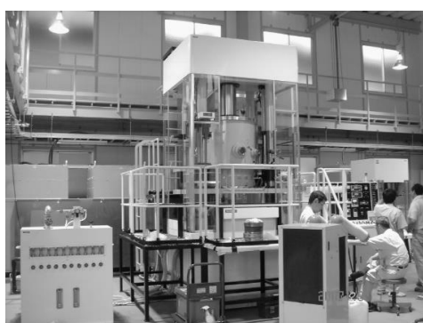
Batch-type Large-size SPS System (Max. pressure 3 MN/pulse current 30,000 A)
