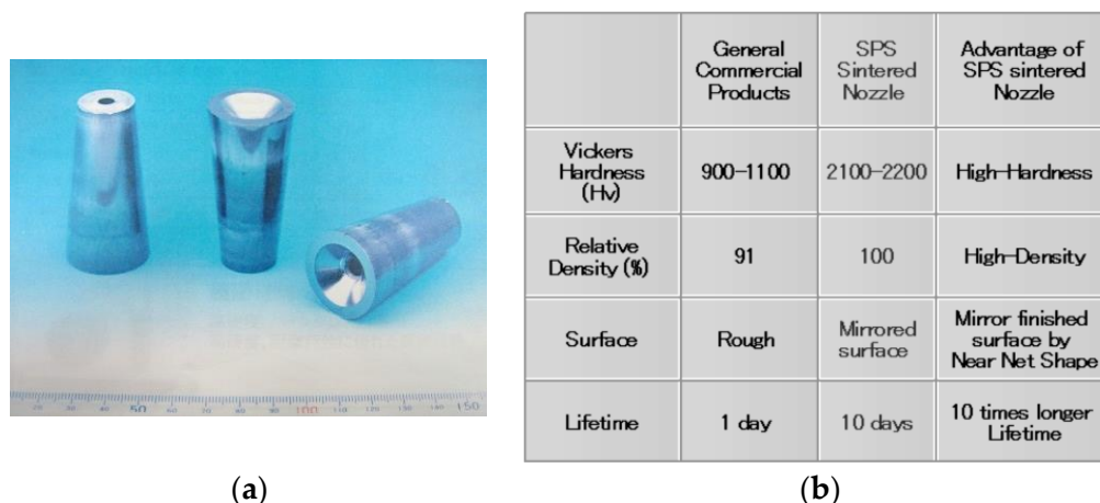
Figure 35. Comparison of SPSed blasting nozzle and other commercial nozzle products: (a) as-sintered SPSed nozzle products: material: \text{Al}_2\text{O}_3 , Length: 60 mm, Outer dia. (Tapered): 30/15 mm, Inner dia. (Straight): 6 mm; (b) Performance comparison table of SPSed \text{Al}_2\text{O}_3 nozzle and other commercial products
