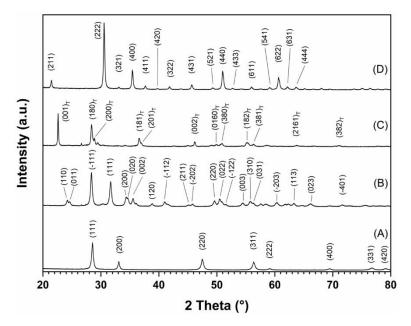
**Figure 2.** XRD patterns of the as-detonated oxide ceramics: (**A**) CeO<sub>2</sub> (JCPDS card No. 01-081-0792), (**B**) HfO<sub>2</sub> (JCPDS card No. 00-034-0104), (**C**) Nb<sub>2</sub>O<sub>5</sub> (JCPDS cards No. 00-30-0873), and (**D**) In<sub>2</sub>O<sub>3</sub> (JCPDS card No. 00-006-0416), respectively.
