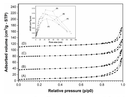
**Figure 4.** Nitrogen isotherms of the as-detonated ceramics: (**A**)  $CeO_2$ , (**B**)  $HfO_2$ , (**C**)  $Nb_2O_5$  and (**D**)  $In_2O_3$  materials, respectively. In the insert, the corresponding particle size distributions.
