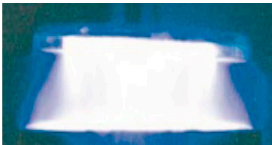
Figure 2. Photograph of the plasma generated by a resistive barrier discharge (RBD) in helium. The gap distance between the electrodes is 4.5 cm, and the voltage is 13 kV RMS at 60 Hz [22]. The input power is around 100 W.
