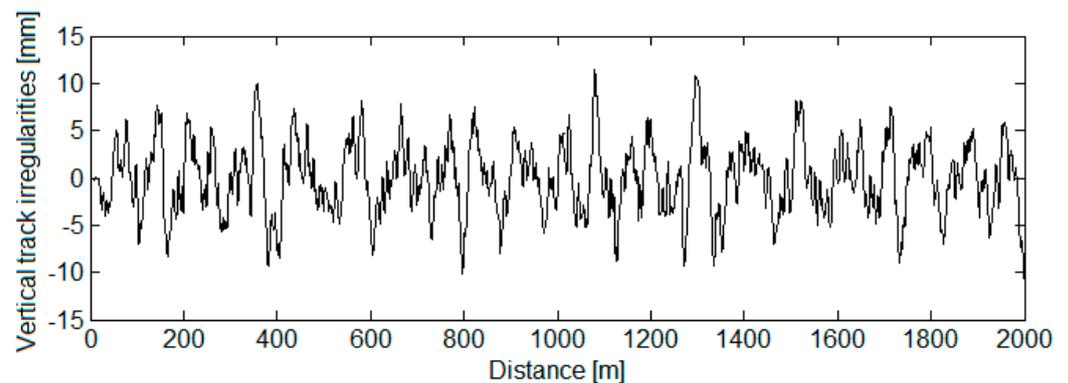
Figure 5. Synthesis of the vertical track irregularities.
