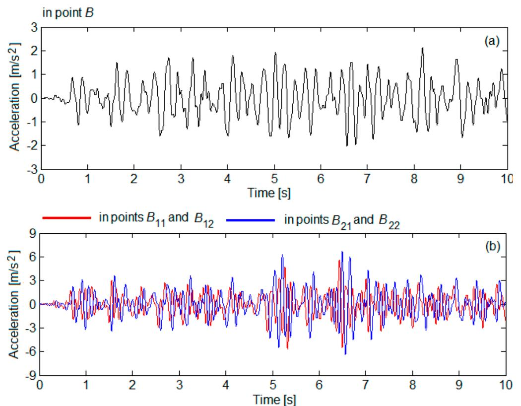
**Figure 6.** Accelerations in the bogie reference points at velocity of 140 km/h (a,b).
