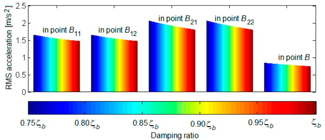
**Figure 8.** Influence the reduction in the damping ratio of suspension upon the RMS acceleration at a velocity of 140 km/h.
