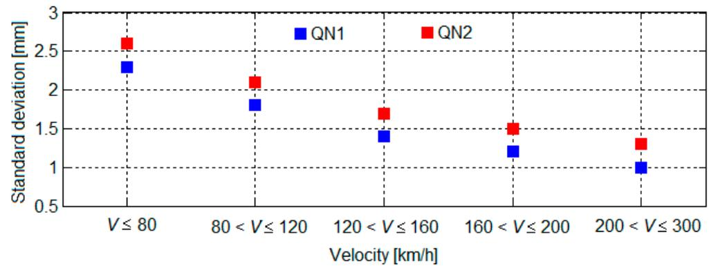
Figure 3. Standard deviations for vertical track irregularities.
