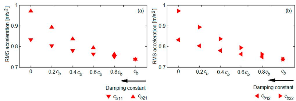
**Figure 10.** Influence the reduction the damping constant of the suspension upon RMS acceleration in point B, at a velocity of 140 km/h: (a) reduction in the damping constant of the suspension in wheels 11 or 12; (b) reduction in the damping constant of the suspension in wheels 21 or 22.
