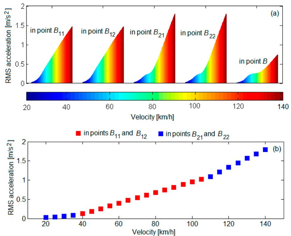
**Figure 7.** RMS acceleration in the bogie reference points: (a) velocity influence upon RMS acceleration; (b) velocity influence upon the critical point of the regime of vibrations of the bogie.
