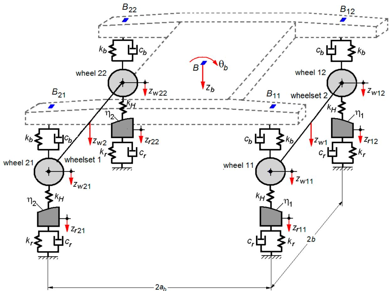
Figure 1. The model of the bogie with symmetrical damping of suspension—track.
