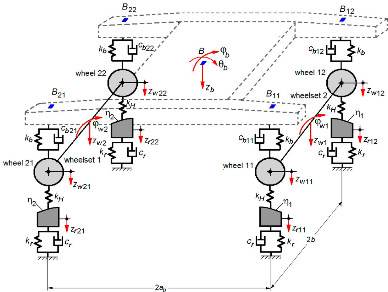
**Figure 2.** The model of the bogie with asymmetrical damping of suspension—track.
