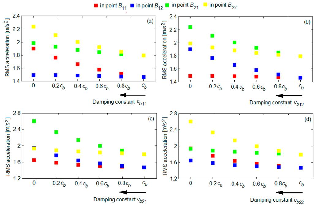
**Figure 9.** Influence the reduction in the damping constant of the suspension upon RMS acceleration at a velocity of 140 km/h: (a) reduction in the damping constant of the suspension of the wheel 11; (b) reduction in the damping constant of the suspension of the wheel 12; (c) reduction in the damping constant of the suspension of the wheel 21; (d) reduction in the damping constant of the suspension of the wheel 22.
