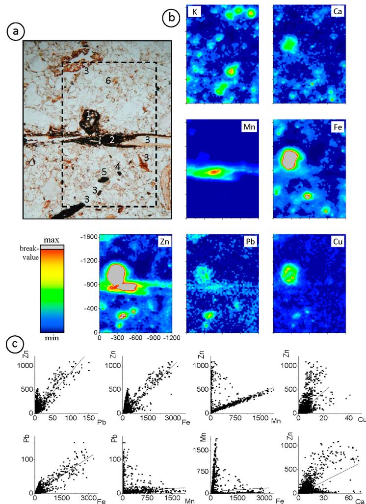
**Figure 2.** Micro X-ray fluorescence analyses in the Ap1 groundmass of a soil under temporary disposal of zinc-smelter waste: (a) optical microscopy image of the analyzed  $1200 \times 1850\text{-}\mu\text{m}$  area: (1) industrial slag fragment; (2) plant root; (3) POM particles; (4) iron oxide; (5) charcoal; and (6) distribution network of the fine soil fraction (plasma); (b) spatial distribution maps of K, Ca, Mn, Fe, Zn, Pb and Cu; and (c) linear regression lines.
