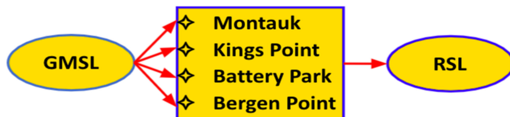
Figure 9. Pathway diagram of the Generalized Additive Model (GAM) to model the relationship between GMSL to RSL (Regional Sea Level) via four regional tidal gauge stations in the New York City and Long Island area.
