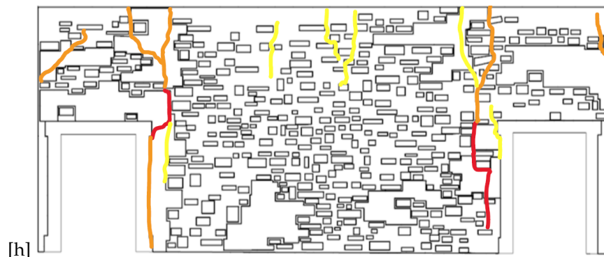
Figure 5. Map of existing cracks on the foundation wall. Red indicates cracking over 1 cm; yellow indicates cracking on the order of 1 mm; orange indicates cracking in between these two limits.
