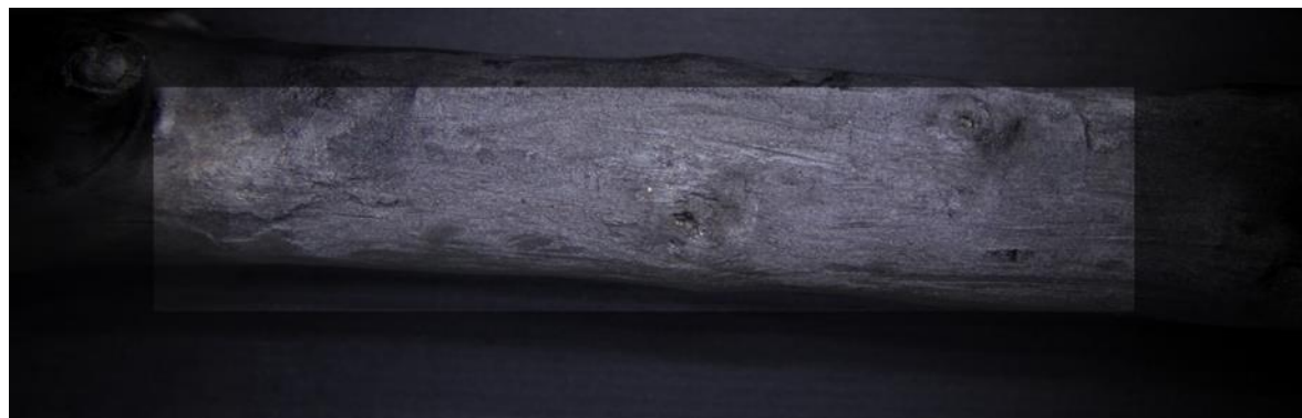
Figure 6. Masking of the region of interest for the application of the Photometric Stereo Imaging (PSI) technique.
