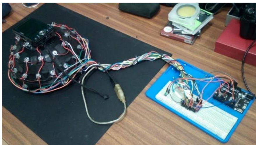
Figure 4. The Reflectance Transformation Imaging (RTI) instrument used in this work.
