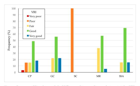
Figure 6. Percentage of Pietra Serena corbels of different qualities according to velocity ratio index (VRI).
