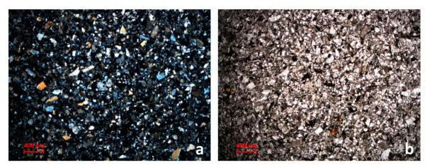
**Figure 3.** (a) GC sample image of the thin section in cross polarized light (xpl); (b) image in plane polarized light (ppl) of the same sample: in both images the medium-fine grain size of quartz and feldspars and the higher compactness of the rock are shown.
