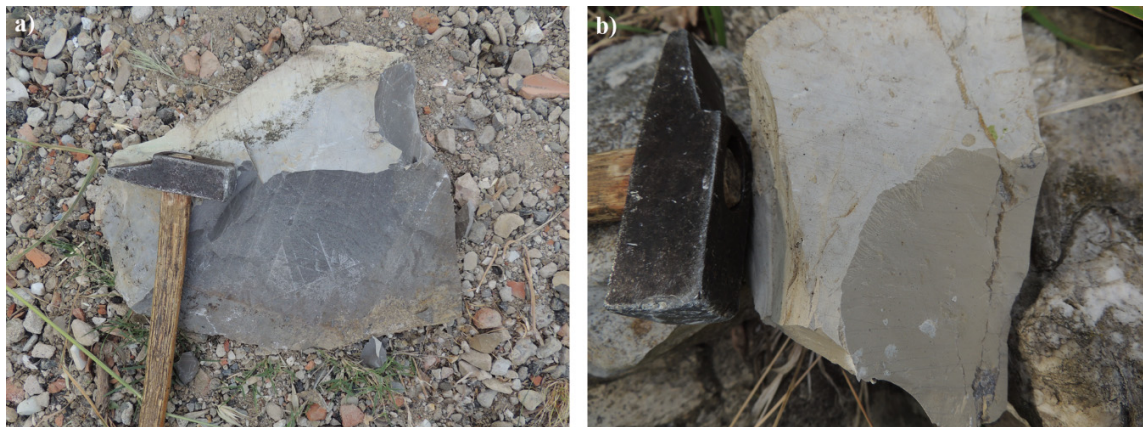
Figure 7. (a) Variety of Pietra Alberese named sasso porcino , dark-colored rock in the fresh cut; (b) variety of Pietra Alberese named sasso alberese , light-colored in fresh cut.
