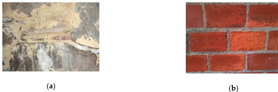
Figure 15. Frost damage on masonry: (a) A layer of ice covering brick inside a church tower. The ice is formed from water-saturated brick and so this effect is not found on the adjacent granite; (b) frost-damaged brick. On some bricks, only the compact surface layer has frozen off, and on others deeper frost damage has resulted in more extensive material loss.
