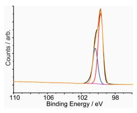
**Figure S1.** Si 2p high resolution spectrum for a freshly prepared Si–H surface, after the etching step. The absence of emission at ~103 eV demonstrates that the starting Si–H surface is free of oxide.
