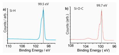
**Figure S2.** XPS analysis showing high resolution Si 2p signal from a pure Si–H surface (a) and a Si surface functionalized with **1**, showing that surface functionalization shifts the Si peak to slightly higher binding energy. All peak energies were calibrated by applying a rigid shift to bring the C 1s emission to 284.7 eV.
