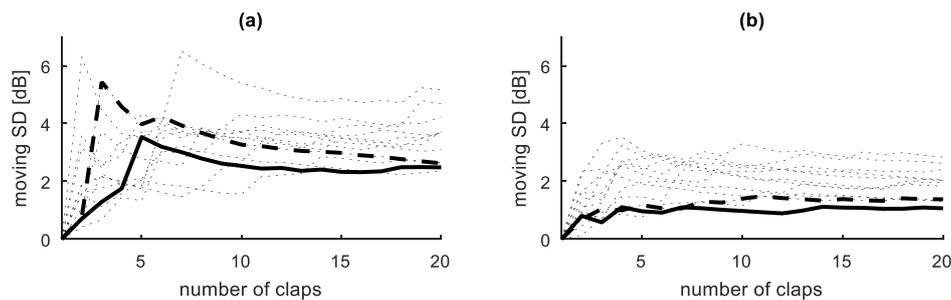
**Figure 4.** Moving standard deviation over the number of handclaps, for all participants, for the 125 Hz octave band. The data of the two participants who have experience in performing room acoustic measurements utilizing handclaps are emphasized with a thicker line type. The left panel (a) gives results without the glove (simple handclap with the A1+ configuration). The right panel (b) gives results for the best fitting glove size per participant (see also Table 2).
