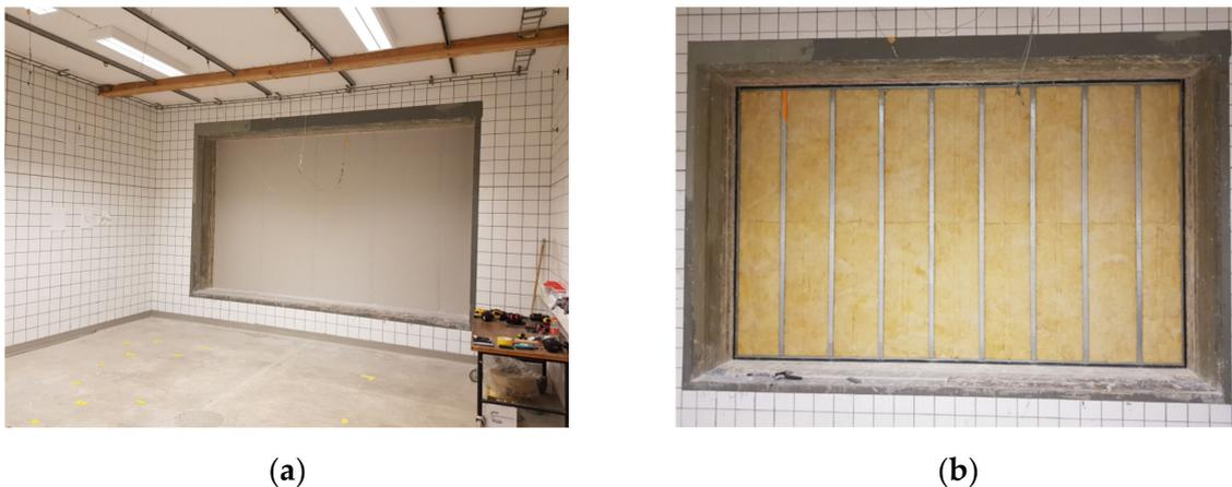
**Figure 2.** Pictures from the measurements of the separating reference wall: (a) The finished mounted wall; (b) The inside of the wall with a sound reduction index of  $R_w$ : 54 dB.
