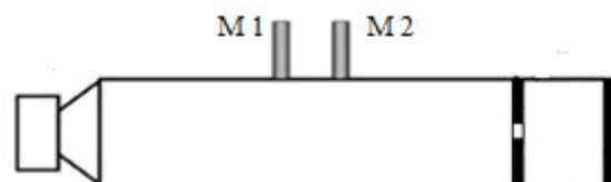
**Figure 4.** Scheme of measurements by the method of two microphones.
