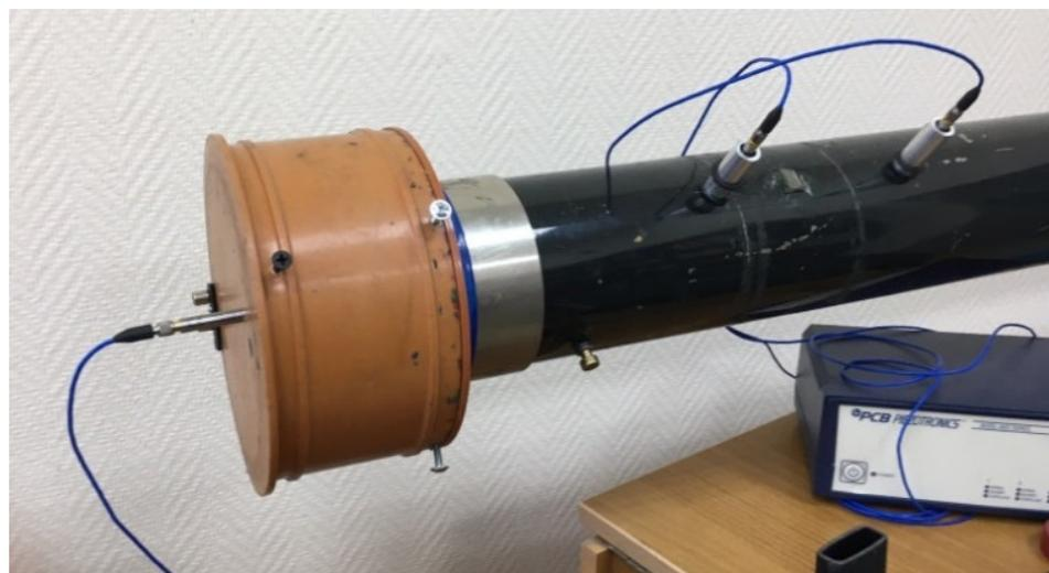
**Figure 5.** View of the measuring setup with an end resonator Helmholtz and three measuring microphones.
