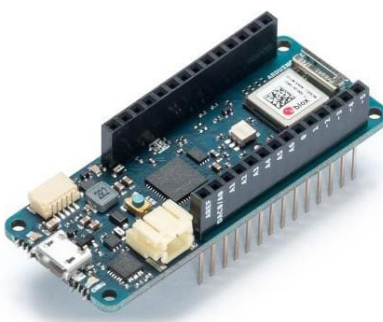
Figure 2. Arduino MKR WIFI 1010 base board.
