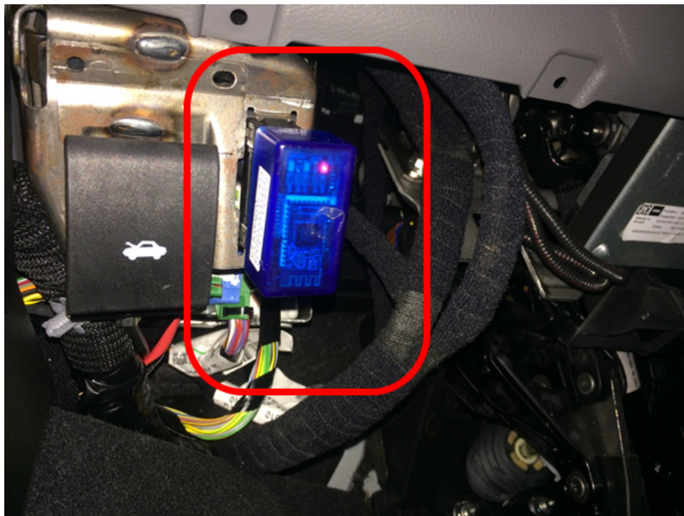
Figure 4. ELM327 connected to a OBD-II interface.
