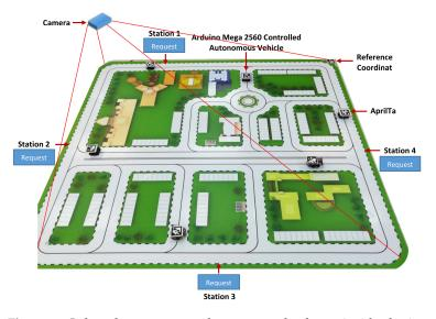
Figure 10. Lab-scale prototype to demonstrate the dynamic ride-sharing system for a smart city.
