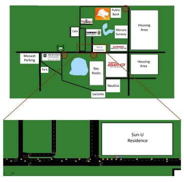
**Figure 4.** Simulation model of the traffic network of Sunway City developed in SUMO with a zoom-in view showing the traffic flow, signalized intersections, and ride-share pick-up location (point B).
