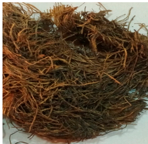
Figure 2. Processed oil palm empty fruit bunch fibres.
