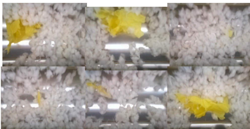
Figure 3. Plastic contamination images, captured by the prototype camera system, as deployed in a commercial cotton gin.
