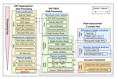
**Figure 2.** Flow-diagram of each of the three image and field sample processing streams. Acronyms: DSM—Digital Surface Model, GCP—Ground Control Point, IGM—Input Geometry Method, SR—Surface Reflectance, Auto ML—Automatic Machine Learning, DSLR—Digital Single-lens Reflex camera, TPOT—Tree-based Pipeline Optimisation Tool, TSDM—Total Standing Dry Matter.
