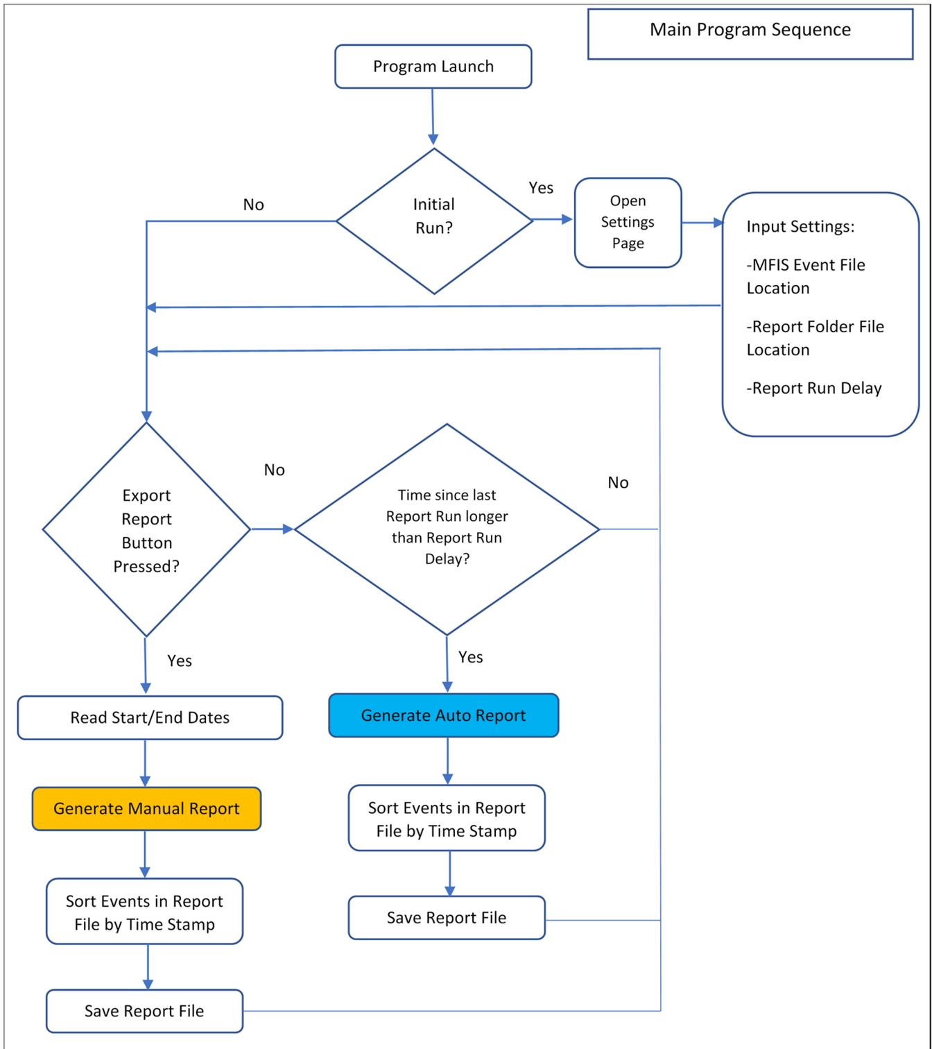
**Figure 9.** Flow chart of the main program sequence for the Inspection Report Builder (IRB) integration software. Sub-processes for generating manual report (shown in orange) and auto report (shown in blue) are detailed in Figures 10 and 11, respectively.
