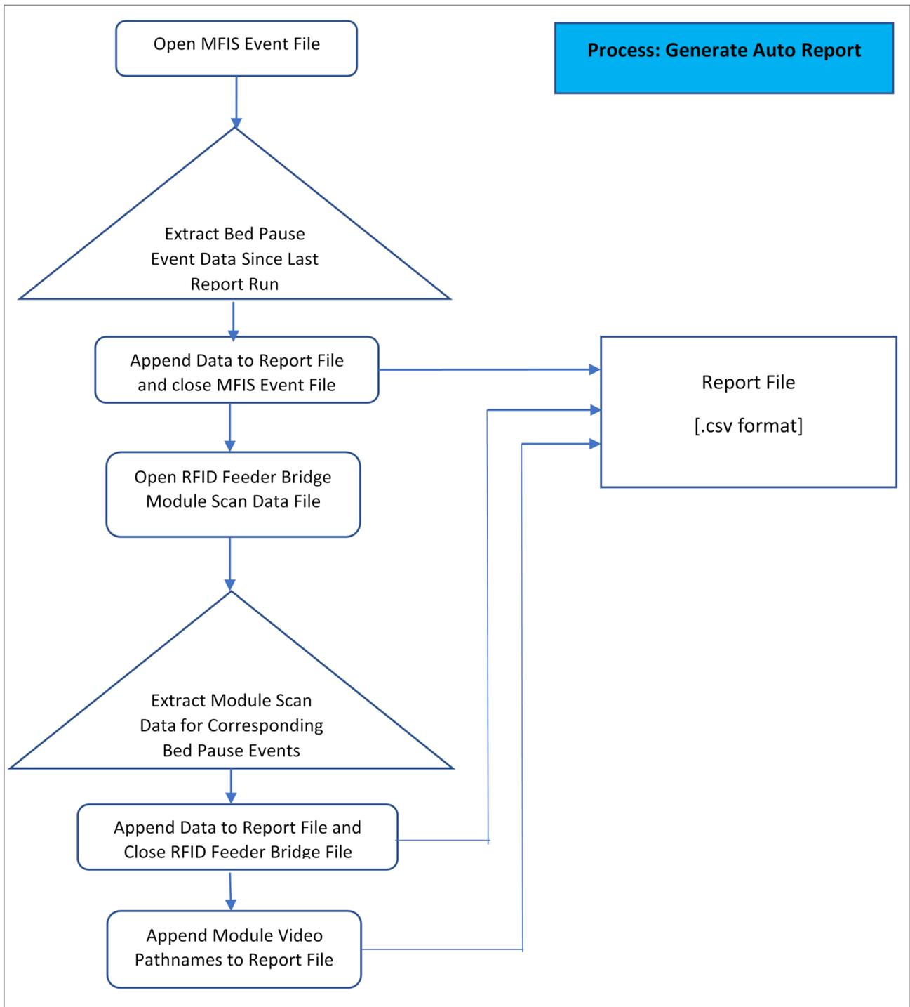
**Figure 11.** Flow chart of the sub-process used to auto-generate a report file from bed pause events stored in the file created by the USDA Module Feeder Inspection system (MFIS) software and the module scan events from the file created by the RFID Feeder Bridge software.
