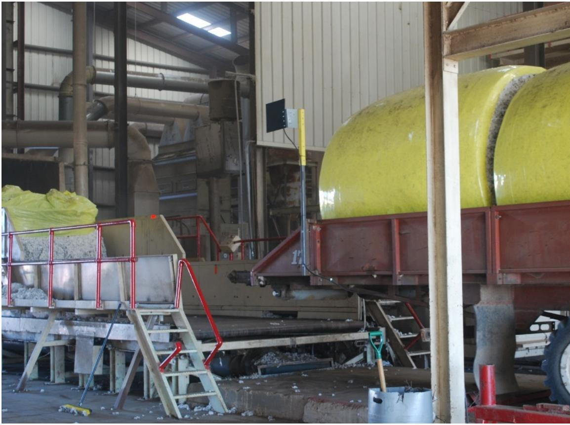
**Figure 2.** Photo of the intake end of a cotton module feeder showing round cotton modules being unloaded from a transport vehicle onto the feeder bed.
