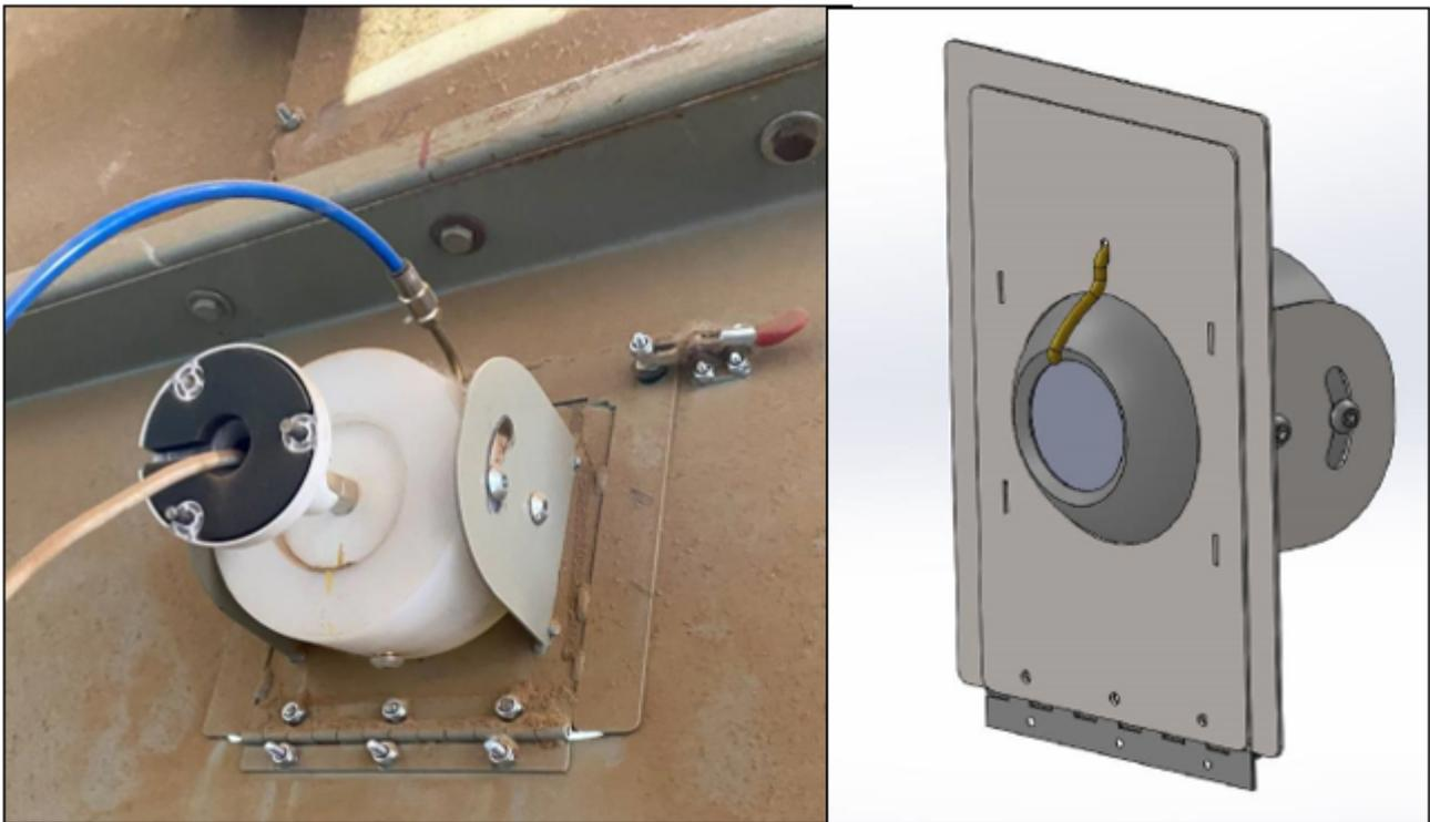
**Figure 5.** Photo (left) and design model (right) of the ball-face camera mounts [13] installed at commercial gin testing locations in 2020.
