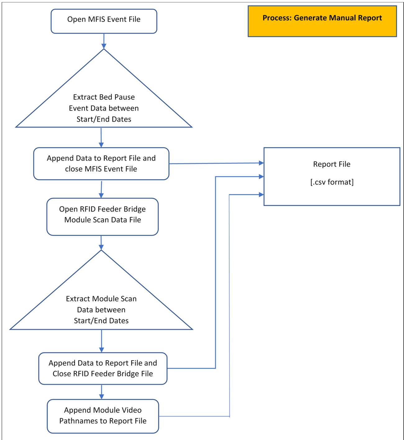
**Figure 10.** Flow chart of the sub-process used to manually generate a report file for a specified time period from bed pause events stored in the file created by the USDA Module Feeder Inspection system (MFIS) software and the module scan events from the file created by the RFID Feeder Bridge software.
