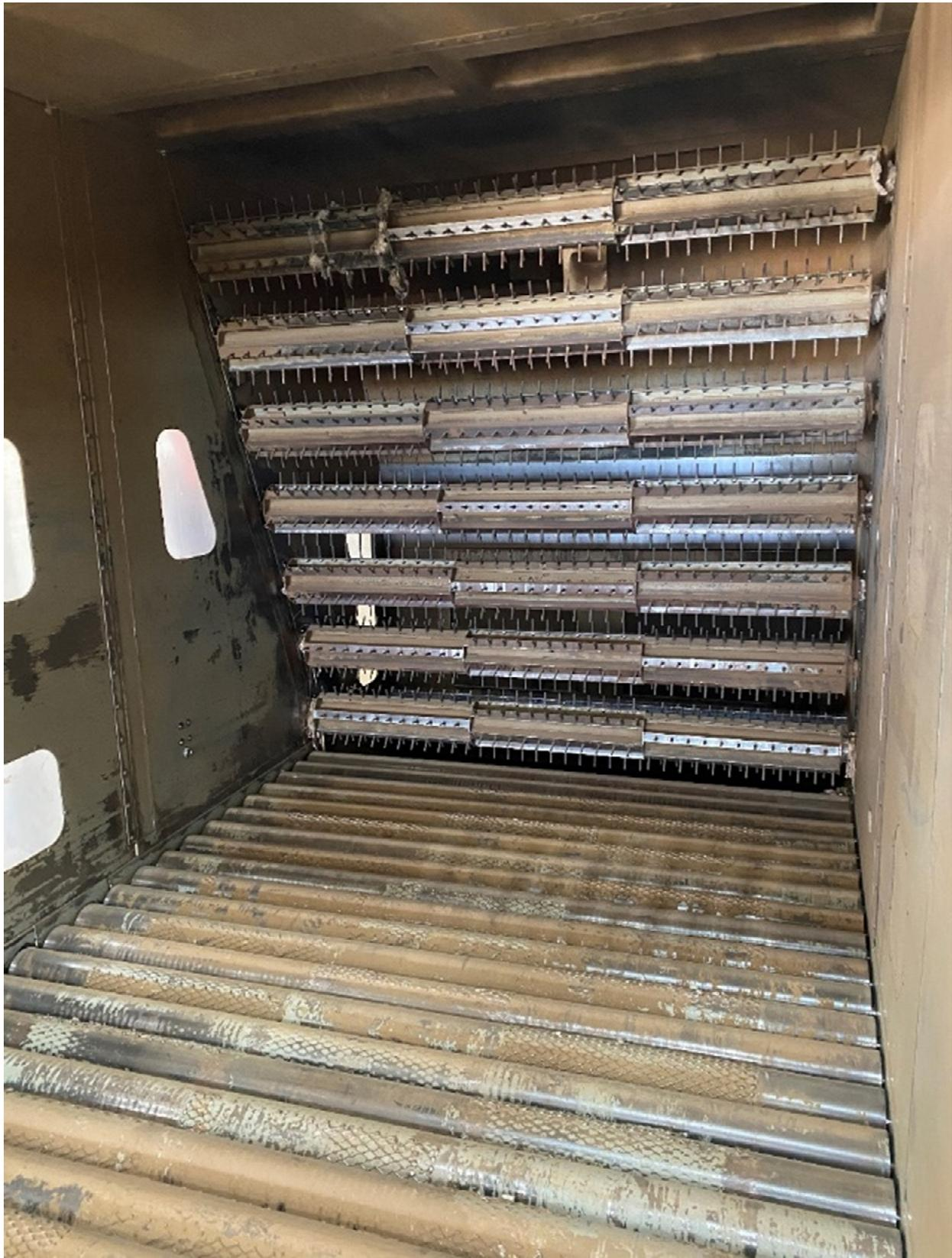
**Figure 1.** Module feeder dispersing cylinders used to break apart cotton modules and feed the material into the ginning process. Dispersing cylinders are approximately 2.75 m long and 46 cm tip to tip diameter covering a total vertical height above the bed rollers of about 3.25 m.
