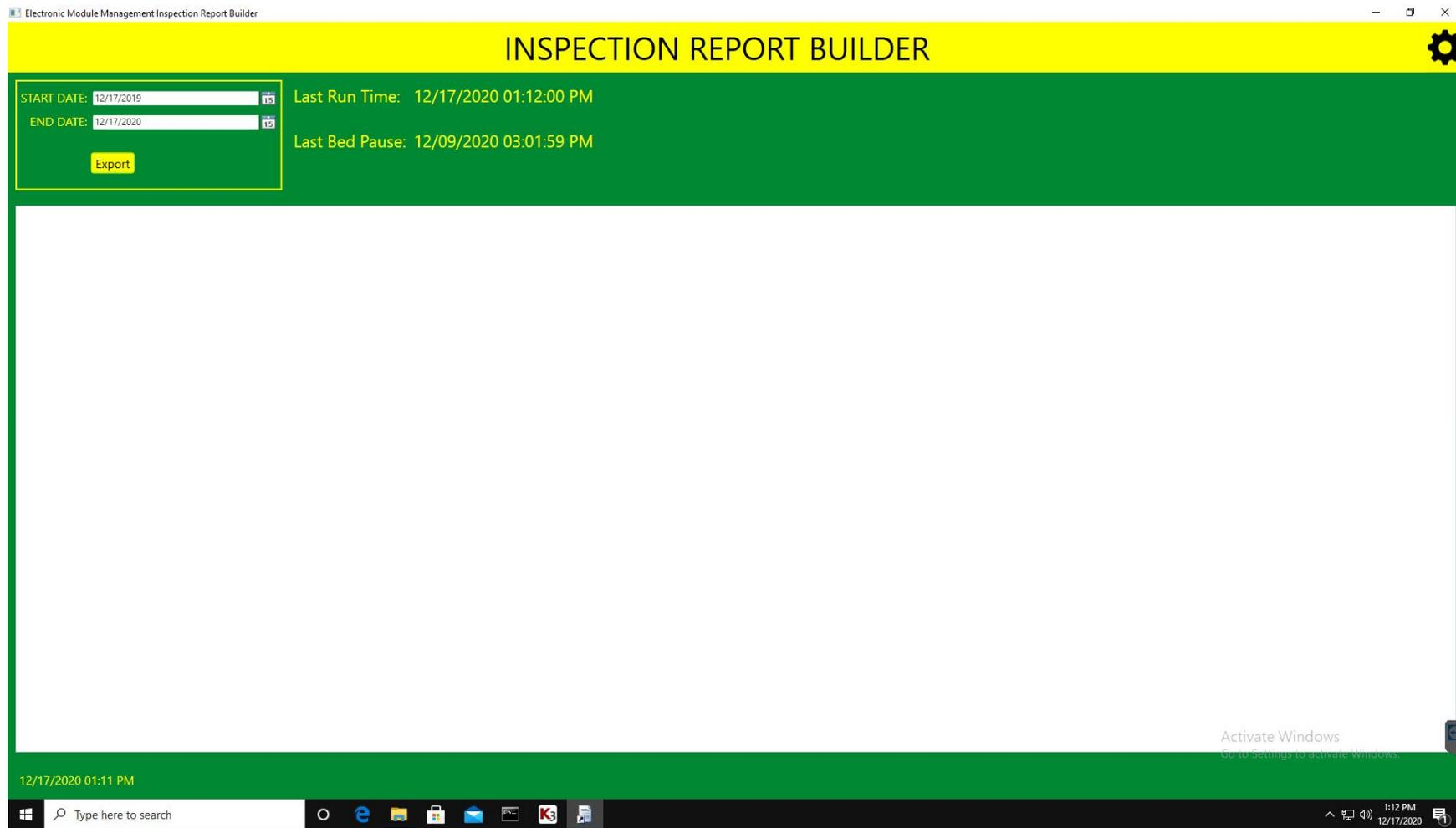
**Figure 7.** Home screen of the Inspection Report Builder software showing user input fields for the desired date range for generation of a manual report and the “last run time” for the most recently automatically generated report.
