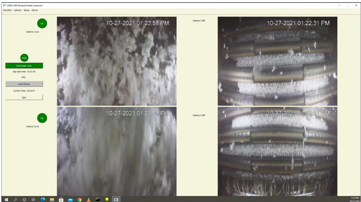
**Figure 6.** USDA Module Feeder Inspection System (MFIS) display showing live video feeds from top and bottom cameras (top and bottom left side images) installed in the dispersing cabinet along with the latest still images (top and bottom right-side images) captured of the dispersing cylinders.
