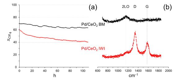
**Figure 6.** (a) Methane conversion in a long-term stability test at 550 °C on Pd/CeO<sub>2</sub> prepared by milling CeO<sub>2</sub> and Pd acetate (5 min at 50 Hz, 0.5 wt.% Pd; Pd/CeO<sub>2</sub> BM) and by incipient wetness impregnation with Pd acetate (Pd/CeO<sub>2</sub> IWI). GHSV =  $12 \times 10^3 h^{-1}$ , F/W = 60 L  $h^{-1} g^{-1}$ . (b) Raman spectra recorded on the samples after reaction.
