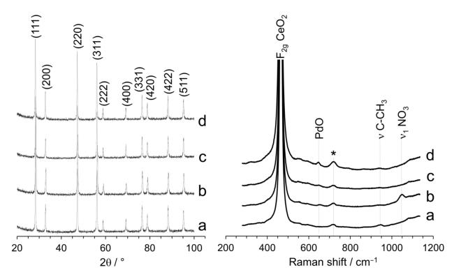
**Figure 2.** XRD profiles and Raman spectra of Pd/CeO<sub>2</sub> catalysts prepared by milling CeO<sub>2</sub> and Pd acetate (**a**) or Pd nitrate (**b**) at 50 Hz for 10 min, and catalysts prepared by incipient wetness impregnation with Pd acetate (**c**) or Pd nitrate (**d**). All catalysts contain a nominal Pd loading of 1 wt.%.
