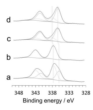
**Figure 3.** Pd 3d X-ray photoelectron spectra of the Pd/CeO<sub>2</sub> catalysts prepared by milling CeO<sub>2</sub> and Pd acetate (**a**) or Pd nitrate (**b**) at 50 Hz for 10 min, and catalysts prepared by incipient wetness impregnation with Pd acetate (**c**) or Pd nitrate (**d**). All catalysts contain a nominal Pd loading of 1 wt.%.
