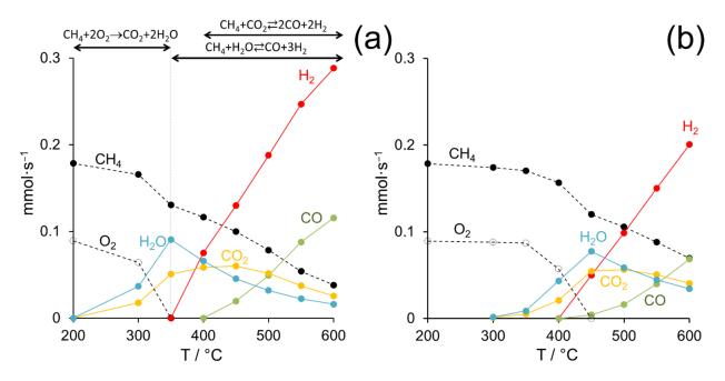
**Figure 4.** Molar flows of the different species present during the partial oxidation of methane on Pd/CeO<sub>2</sub> (0.5 wt.% Pd) prepared by dry ball milling from palladium acetate and CeO<sub>2</sub> at 50 Hz for 5 min (**a**) and by incipient wetness impregnation of CeO<sub>2</sub> with Pd acetate (**b**). GHSV =  $12 \times 10^3$  h<sup>-1</sup>, F/W = 60 L h<sup>-1</sup> g<sup>-1</sup>.
