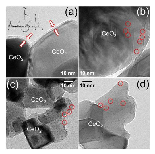
**Figure 1.** HRTEM images of the Pd/CeO<sub>2</sub> catalysts prepared by milling CeO<sub>2</sub> and Pd acetate (**a**) or Pd nitrate (**b**) at 50 Hz for 10 min, and catalysts prepared by incipient wetness impregnation with Pd acetate (**c**) or Pd nitrate (**d**). All catalysts contain a nominal Pd loading of 1 wt.%.
