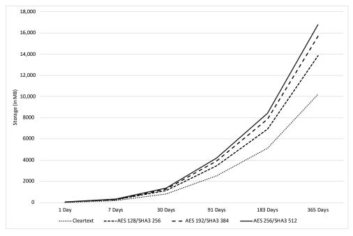
Figure 5. Storage requirements per key size.
