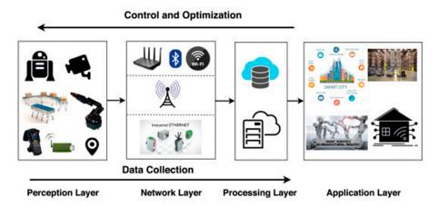
Figure 1. Generalised IIoT system architecture.
