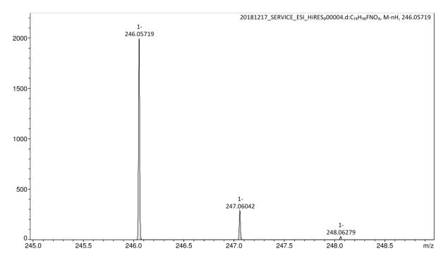
Figure 24. HR-MS (ESI<sup>+</sup>) of N-(4-fluorophenyl)-2,5-dihydroxybenzamide.
