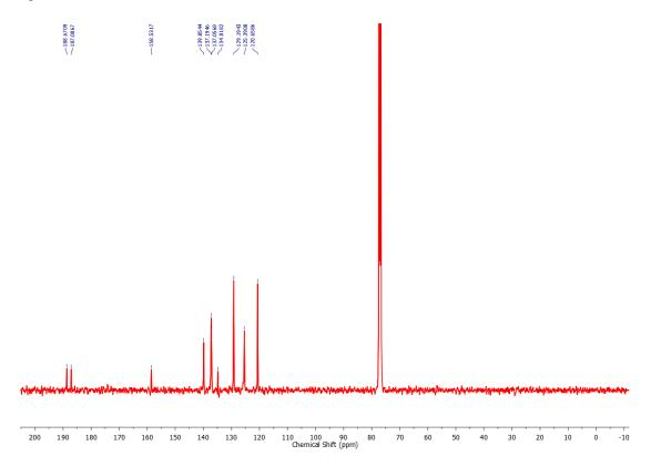
Figure 30.  ${}^{13}C{}^{1}H$  NMR (101 MHz) spectrum of 3,6-dioxo-*N*-phenylcyclohexa-1,4-diene-1-carboxamide in CDCl<sub>3</sub> at 298 K.
