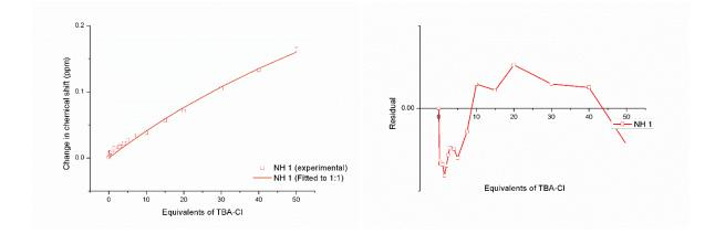
Figure 48. Fitted binding isotherm of 2,5-dimethoxy-N-(p-tolyl)benzamide + TBACl showing the change in chemical shift of the NH proton fitted to the 1:1 binding model (left).  $K_a = 1.48 \text{ M}^{-1}$  Residual plot showing the random error obtained from the binding isotherm fitting (right). Covariance of fit (cov<sub>fit</sub>) = 5.34 x 10<sup>-3</sup>. Link to Bindfit fitting: http://app.supramolecular.org/bindfit/view/6f20ff00-a6c8-4bd6-9451-accc783b3fb0.
