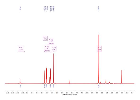
Figure 33. <sup>1</sup>H NMR (400 MHz) spectrum of 3,6-dioxo-N-(p-tolyl)cyclohexa-1,4-diene-1-carboxamide in CDCl<sub>3</sub> at 298 K.
