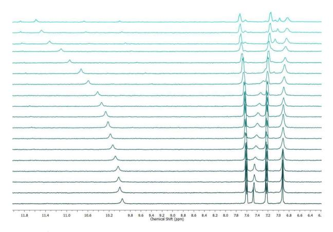
Figure 69. <sup>1</sup>H NMR titration spectra as a stack plot for 3,6-dioxo-N-(p-tolyl)cyclohexa-1,4-diene-1carboxamide (5 mM) + TBACl in  $CD_3CN-d_3$  at 298 K.
