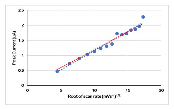
Figure 80. Plot of the root of scan rate  $(v^{1/2})$  against peak current  $(I_{p,c})$  for compound 5 3,6dioxo-*N*-phenylcyclohexa-1,4-diene-1-carboxamide. The red line shows the line of best fit through the origin, the blue line shows the true line of best fit.
