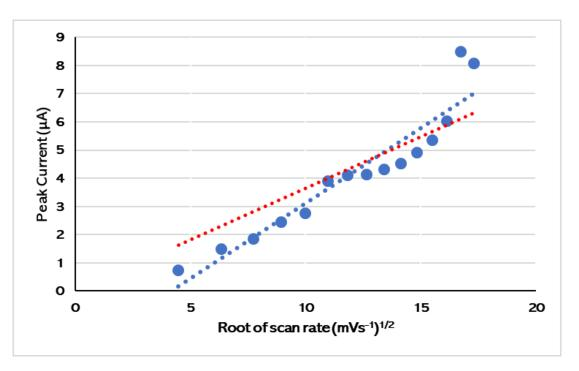
Figure 86. Plot of the root of scan rate  $(v^{1/2})$  against peak current  $(I_{p,c})$  for **8** *N*-(3,5-bis(trifluoromethyl)phenyl)-3,6-dioxocyclohexa-1,4-diene-1-carboxamide. The red line shows the line of best fit through the origin, the blue line shows the true line of best fit.
