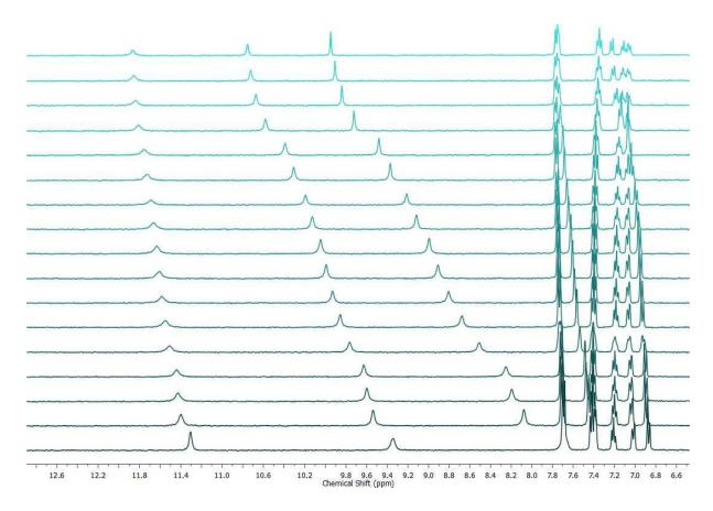
Figure 53. <sup>1</sup>H NMR titration spectra as a stack plot for 2,5-dihydroxy-*N*-phenylbenzamide (5 mM) + TBACl in CD<sub>3</sub>CN-d<sub>3</sub> /1% DMSO- $d_6$  at 298 K.
