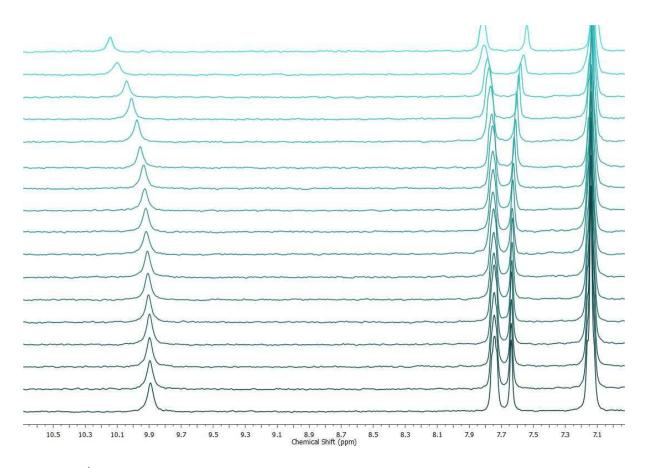
Figure 49. <sup>1</sup>H NMR titration spectra as a stack plot for *N*-(4-fluorophenyl)-2,5-dimethoxybenzamide (5 mM) + TBACl in CD<sub>3</sub>CN-d<sub>3</sub> /1% DMSO- $d_6$  at 298 K.
