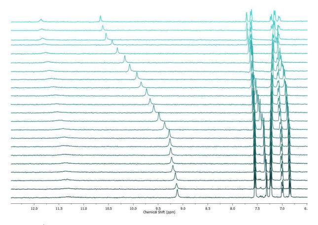
Figure 56. <sup>1</sup>H NMR titration spectra as a stack plot for 2,5-dihydroxy-N-(p-tolyl)benzamide (5 mM) + TBACl in CD<sub>3</sub>CN-d<sub>3</sub> /1% DMSO- $d_6$  at 298 K.
