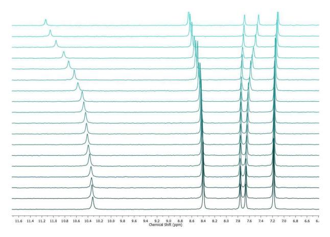
Figure 51. <sup>1</sup>H NMR titration spectra as a stack plot for N-(3,5-bis(trifluoromethyl)phenyl)-2,5-dimethoxybenzamide (5 mM) + TBACl in CD<sub>3</sub>CN-d<sub>3</sub>/1% DMSO-d<sub>6</sub> at 298 K.
