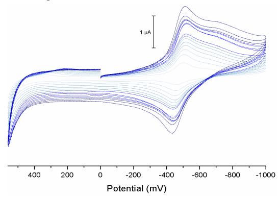
Figure 79. Series of cyclic voltammograms of compound **5** 3,6-dioxo-*N*-phenylcyclohexa-1,4-diene-1-carboxamide taken from scan rate  $20 \text{ mVs}^{-1}$  to  $300 \text{ mVs}^{-1}$ . The current response increases with faster scan rates.
