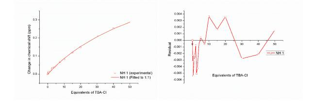
Figure 50. Fitted binding isotherm of N-(4-fluorophenyl)-2,5-dimethoxybenzamide + TBACl showing the change in chemical shift of the NH proton fitted to the 1:1 binding model (left).  $K_a = 2.92 \text{ M}^{-1}$  Residual plot showing the random error obtained from the binding isotherm fitting (right). Covariance of fit (cov<sub>fit</sub>) = 8.91 x 10<sup>-4</sup>. Link to Bindfit fitting: http://app.supramolecular.org/bindfit/view/5bfbd64f-7e92-4de1-8492-aa930d7321dc.
