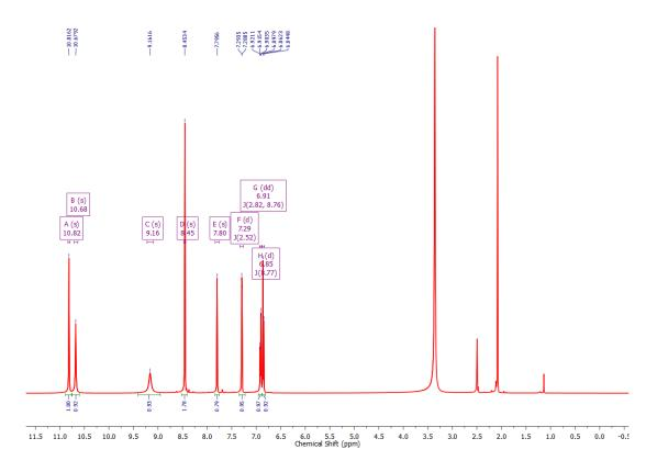
Figure 25. <sup>1</sup>H NMR (500 MHz) spectrum of N-(3,5-bis(trifluoromethyl)phenyl)-2,5dimethoxybenzamide in  $(CD_3)_2SO$  at 298 K.
