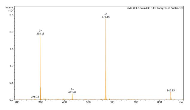
Figure 7. LR-MS (ESI<sup>+</sup>) of N-(4-fluorophenyl)-2,5-dimethoxybenzamide.
