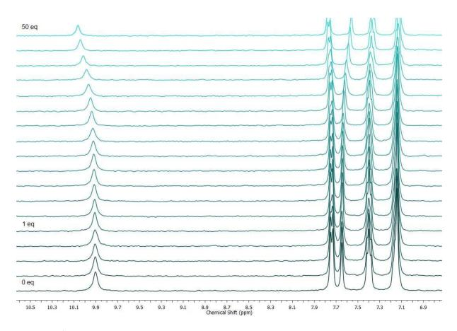
Figure 45. <sup>1</sup>H NMR titration spectra as a stack plot for 2,5-dimethoxy-N-phenylbenzamide (5 mM) + TBACl in  $CD_3CN-d_3 / 1\%$  DMSO- $d_6$  at 298 K.
