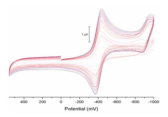
Figure 81. Series of cyclic voltammograms of compound **6** 3,6-dioxo-N-(p-tolyl)cyclohexa-1,4-diene-1-carboxamide taken from scan rate 20 mVs<sup>-1</sup> to 300 mVs<sup>-1</sup>. The current response increases with faster scan rates.
