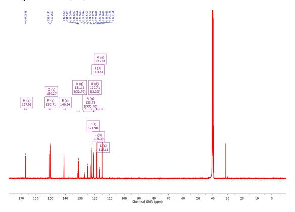
Figure 26.  ${}^{13}C{}^{1}H$  NMR (101 MHz) spectrum of N-(3,5-bis(trifluoromethyl)phenyl)-2,5-dimethoxybenzamide in (CD<sub>3</sub>)<sub>2</sub>SO at 298 K.
