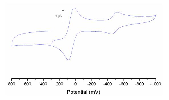
Figure 77. Cyclic Voltammogram of compound **7** N-(4-fluorophenyl)-3,6-dioxocyclohexa-1,4-diene-1-carboxamide at 100 mVs<sup>-1</sup> in the presence of Fc/Fc<sup>+</sup>.
