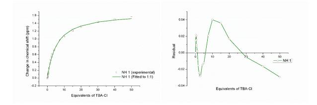
Figure 57. Fitted binding isotherm of N-(4-fluorophenyl)-2,5-dihydroxybenzamide + TBACl showing the change in chemical shift of the OH and NH protons fitted to the 1:1 binding model (left)  $K_a = 41.47$ M<sup>-1</sup>. Residual plot showing the random error obtained from the binding isotherm fitting (right). 10-3. Covariance of 1.56 fit (cov<sub>fit</sub>) = х Link to Bindfit fitting: http://app.supramolecular.org/bindfit/view/d28e7bd7-dbf9-4532-851d-7a81ca565211.
