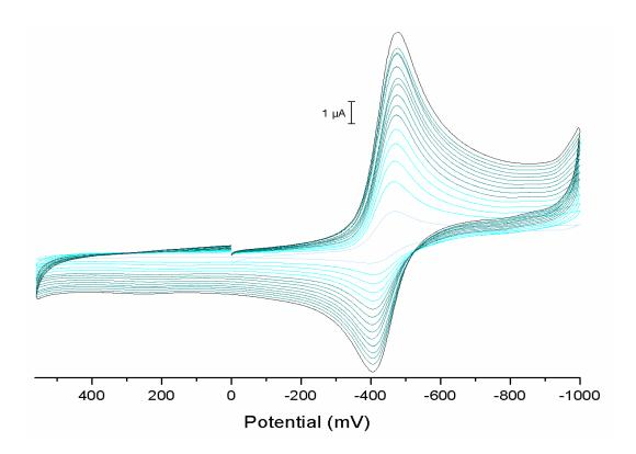
Figure 83. Series of cyclic voltammograms of compound 7 N-(4-fluorophenyl)-3,6-dioxocyclohexa-1,4-diene-1-carboxamide taken from scan rate 20 mVs<sup>-1</sup> to 300 mVs<sup>-1</sup>. The current response increases with faster scan rates.
