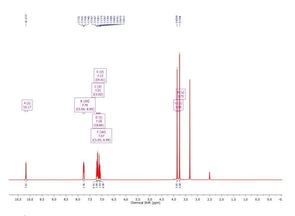
Figure 5. <sup>1</sup>H NMR (500 MHz) spectrum of N-(4-fluorophenyl)-2,5-dimethoxybenzamide in (CD<sub>3</sub>)<sub>2</sub>SO<sub>3</sub> at 298 K.
