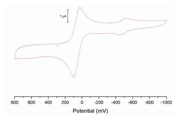
Figure 76. Cyclic Voltammogram of compound **6** 3,6-dioxo-N-(p-tolyl)cyclohexa-1,4-diene-1- carboxamide at  $100 \text{ mVs}^{-1}$  in the presence of Fc/Fc<sup>+</sup>.
