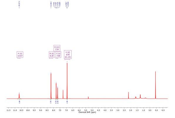
Figure 41. <sup>1</sup>H NMR (400 MHz) spectrum of N-(3,5-bis(trifluoromethyl)phenyl)-3,6-dioxocyclohexa-1,4-diene-1-carboxamide in CDCl<sub>3</sub> at 298 K.
