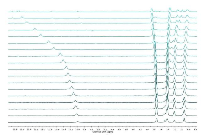
Figure 65. <sup>1</sup>H NMR titration spectra as a stack plot for 3,6-dioxo-*N*-phenylcyclohexa-1,4-diene-1carboxamide (5 mM) + TBACl in CD<sub>3</sub>CN-d<sub>3</sub> /1% DMSO- $d_6$  at 298 K.
