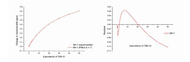
Figure 52. Fitted binding isotherm of N-(3,5-bis(trifluoromethyl)phenyl)-2,5-dimethoxybenzamide + TBACl showing the change in chemical shift of the NH proton fitted to the 1:1 binding model (left). Ka =  $6.69 \text{ M}^{-1}$  Residual plot showing the random error obtained from the binding isotherm fitting (right). 10-3. 1.16 Covariance of fit (cov<sub>fit</sub>) = Х Link to Bindfit fitting: http://app.supramolecular.org/bindfit/view/e6081634-e1d0-49a8-a641-7e7c69fd6d15.
