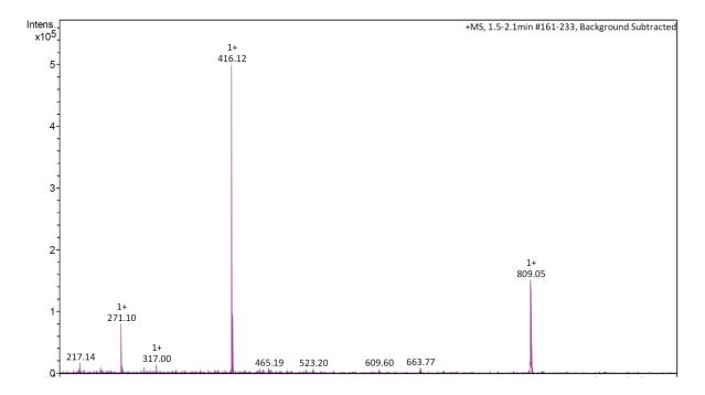
Figure 11. LR-MS (ESI<sup>+</sup>) of N-(3,5-bis(trifluoromethyl)phenyl)-2,5-dimethoxybenzamide.
