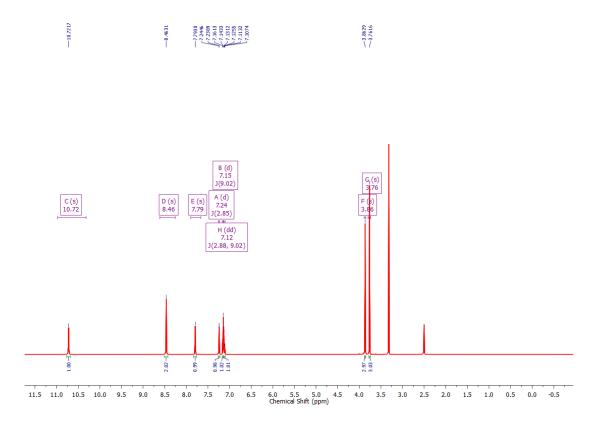
Figure 9. <sup>1</sup>H NMR (500 MHz) spectrum of N-(3,5-bis(trifluoromethyl)phenyl)-2,5-dimethoxybenzamide in (CD<sub>3</sub>)<sub>2</sub>SO at 298 K.
