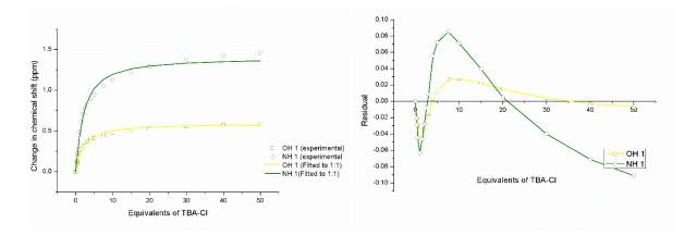
Figure 60. Fitted binding isotherm of N-(4-fluorophenyl)-2,5-dihydroxybenzamide + TBACl showing the change in chemical shift of the OH and NH protons fitted to the 1:1 binding model (left)  $K_a = 125.55$ M<sup>-1</sup>. Residual plot showing the random error obtained from the binding isotherm fitting (right). 9.07 10-3. Covariance of fit  $(cov_{fit})$ = х Link to Bindfit fitting: http://app.supramolecular.org/bindfit/view/d1dfa649-4fa8-4dc9-9486-54fa7b6dc005.
