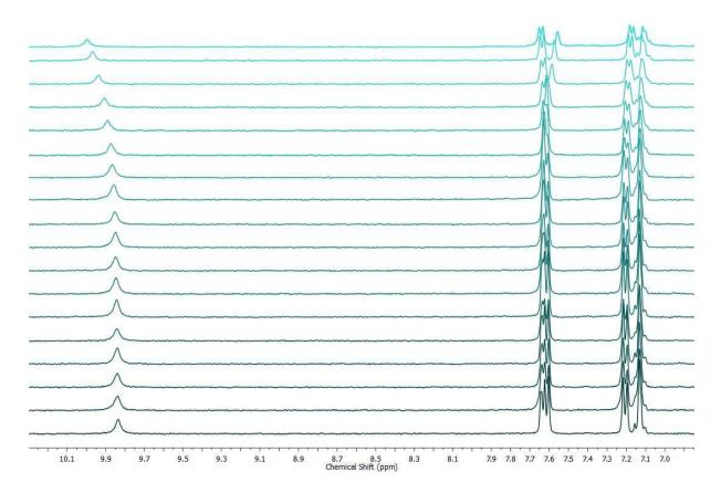
Figure 47. <sup>1</sup>H NMR titration spectra as a stack plot for 2,5-dimethoxy-N-(p-tolyl)benzamide (5 mM) + TBACl in CD<sub>3</sub>CN-d<sub>3</sub> /1% DMSO- $d_6$  at 298 K.
