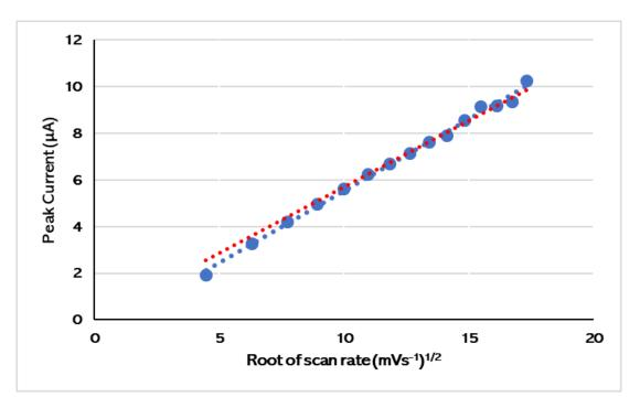
Figure 84. Plot of the root of scan rate ( $v^{1/2}$ ) against peak current ( $I_{p,c}$ ) for **7** *N*-(4-fluorophenyl)-3,6-dioxocyclohexa-1,4-diene-1-carboxamide. The red line shows the line of best fit through the origin, the blue line shows the true line of best fit.
