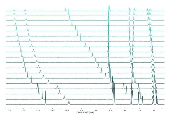
Figure 62. <sup>1</sup>H NMR titration spectra as a stack plot for N-(3,5-bis(trifluoromethyl)phenyl)-2,5-dihydroxybenzamide (5 mM) + TBACl in CD<sub>3</sub>CN-d<sub>3</sub> /1% DMSO-d<sub>6</sub> at 298 K.
