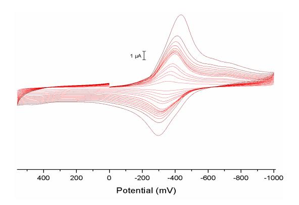
Figure 85. Series of cyclic voltammograms of compound **8** N-(3,5-bis(trifluoromethyl)phenyl)-3,6-dioxocyclohexa-1,4-diene-1-carboxamide taken from scan rate 20 mVs<sup>-1</sup> to 300 mVs<sup>-1</sup>. The current response increases with faster scan rates.
