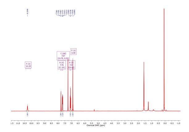
Figure 37. <sup>1</sup>H NMR (400 MHz) spectrum of N-(4-fluorophenyl)-3,6-dioxocyclohexa-1,4-diene-1-carboxamide in CDCl<sub>3</sub> at 298 K.
