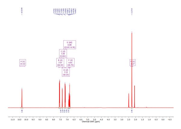
Figure 17. <sup>1</sup>H NMR (400 MHz) spectrum of 2,5-dihydroxy-N-(p-tolyl)benzamide in (CD<sub>3</sub>)<sub>2</sub>SO at 298 K.
