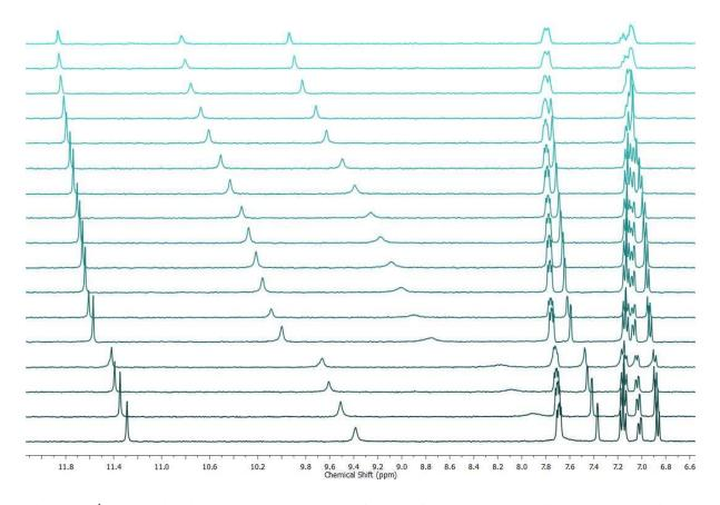
Figure 59. <sup>1</sup>H NMR titration spectra as a stack plot for *N*-(4-fluorophenyl)-2,5-dihydroxybenzamide (5 mM) + TBACl in CD<sub>3</sub>CN-d<sub>3</sub>/1% DMSO- $d_6$  at 298 K.
