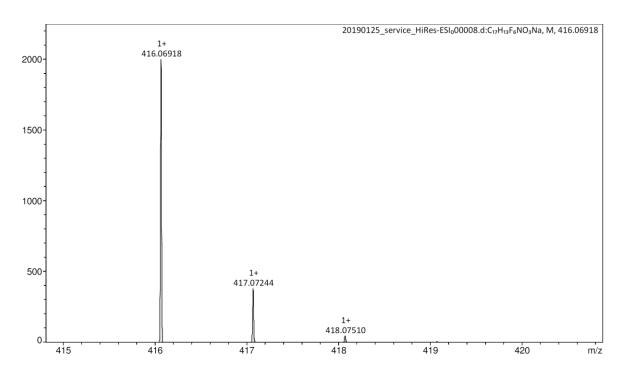
Figure 12. HR-MS (ESI<sup>+</sup>) of *N*-(3,5-bis(trifluoromethyl)phenyl)-2,5-dimethoxybenzamide.
