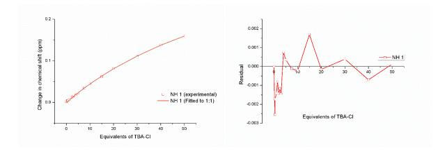
Figure 46. Fitted binding isotherm of 2,5-dimethoxy-N-phenylbenzamide + TBACl showing the change in chemical shift of the NH proton fitted to the 1:1 binding model (left).  $K_a = 2.18 \text{ M}^{-1}$  Residual plot showing the random error obtained from the binding isotherm fitting (right). Covariance of fit (cov<sub>fit</sub>) = 4.57 x 10<sup>-4</sup>. Link to Bindfit fitting: http://app.supramolecular.org/bindfit/view/a3a8083e-2d82-4ce7-8eb8-8c326a21b893.
