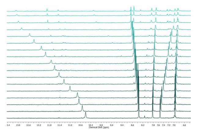
Figure 73. <sup>1</sup>H NMR titration spectra as a stack plot for N-(3,5-bis(trifluoromethyl)phenyl)-3,6-dioxocyclohexa-1,4-diene-1-carboxamide (5mM) + TBACl in CD<sub>3</sub>CN-d<sub>3</sub> at 298 K.
