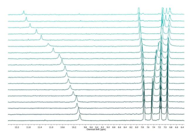
Figure 71. <sup>1</sup>H NMR titration spectra as a stack plot for *N*-(4-fluorophenyl)-3,6-dioxocyclohexa-1,4-diene-1-carboxamide (5mM) + TBACl in CD<sub>3</sub>CN-d<sub>3</sub> at 298 K.
