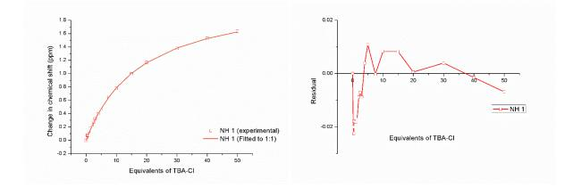
Figure 70. Fitted binding isotherm of 3,6-dioxo-N-(p-tolyl)cyclohexa-1,4-diene-1-carboxamide + TBACl showing the change in chemical shift of the NH proton fitted to the 1:1 binding model (left). Ka =  $11.39 \text{ M}^{-1}$  Residual plot showing the random error obtained from the binding isotherm fitting (right). 10-4. 3.79 Covariance of fit (cov<sub>fit</sub>) = х Link to Bindfit fitting: http://app.supramolecular.org/bindfit/view/702ba05b-af22-41f8-92d3-03851c9bbfa4.
