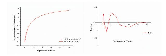
Figure 58. Fitted binding isotherm of 2,5-dihydroxy-N-(p-tolyl)benzamide + TBACl showing the change in chemical shift of the NH protons fitted to the 2:1 binding model (left)  $K_{11} = 191.36 \text{ M}^{-1}$ ,  $K_{12}$ = 665.6 M<sup>-1</sup>.Residual plot showing the random error obtained from the binding isotherm fitting (right). 10-4. Covariance of fit (cov<sub>fit</sub>) 1.28 Link Bindfit fitting: = х to http://app.supramolecular.org/bindfit/view/7a990a8d-730c-4de2-b904-2821f4114c32.
