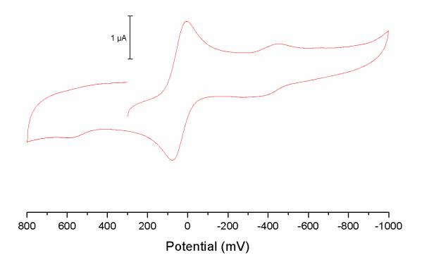
Figure 78. Cyclic Voltammogram of compound **8** N-(3,5-bis(trifluoromethyl)phenyl)-3,6-dioxocyclohexa-1,4-diene-1-carboxamide at 100 mVs<sup>-1</sup> in the presence of Fc/Fc<sup>+</sup>.
