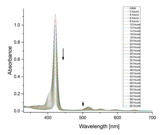
**Figure 2.** Changes in the absorption of porphyrin 1 observed upon irradiation. The sample was irradiated for 60 h, using an LED emitting at 420 nm (63 mW).
