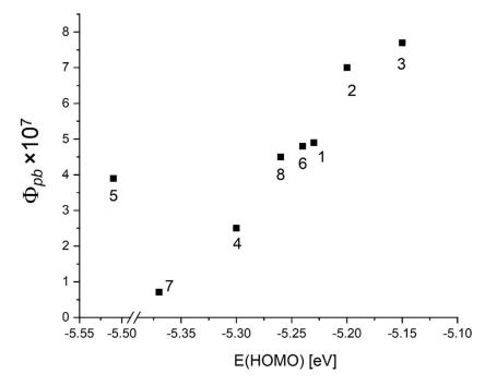
**Figure 4.** Correlation between the observed photobleaching quantum yields and the calculated highest occupied molecular orbital (HOMO) energies.
