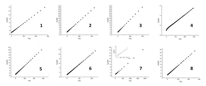
**Figure 3.** The ratio of the initial absorption,  $A_0$ , to the absorption recorded after irradiating for time *t*, A(t), vs. F(t), obtained for the toluene solutions of porphyrins 1–8 at 293 K. The monitoring wavelengths correspond to the absorption maxima (see Table 1). The inset shows deviation from linearity in the initial period of irradiation of porphyrin 7.
