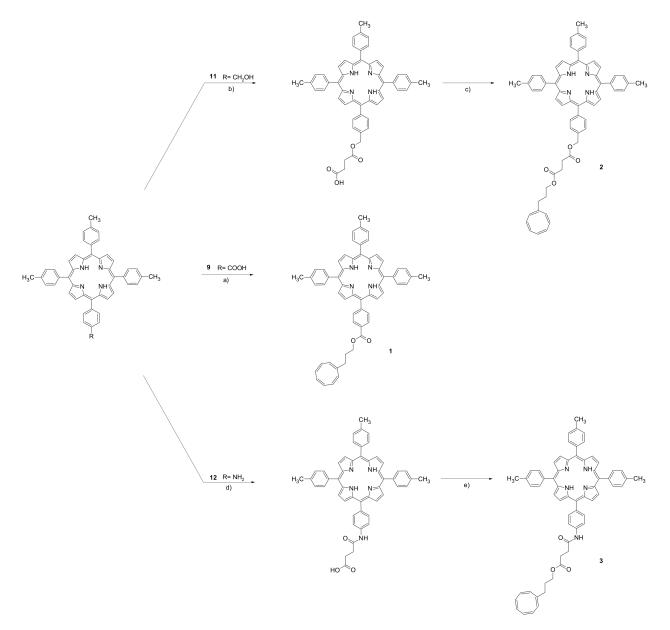
**Scheme 3.** Syntheses of porphyrins containing one cyclooctatetraene (COT) moiety. Reagents and conditions: (a) 1,3,5,7-cyclooctatetraene-1-propanol (COT-OH), 4-DMAP, EDCI.Cl, anhydrous THF, rt, overnight; 49%. (b) succinic anhydride, Et<sub>3</sub>N, anhydrous DCM, rt, 16 h; 48%. (c) COT-OH, 4-DMAP, EDCI.Cl, anhydrous THF, rt, overnight; 55% (d) succinic anhydride, Et<sub>3</sub>N, anhydrous DCM, rt, 16 h; 83%. (e) COT-OH, 4-DMAP, EDCI.Cl, anhydrous THF, rt, overnight; 53%.
