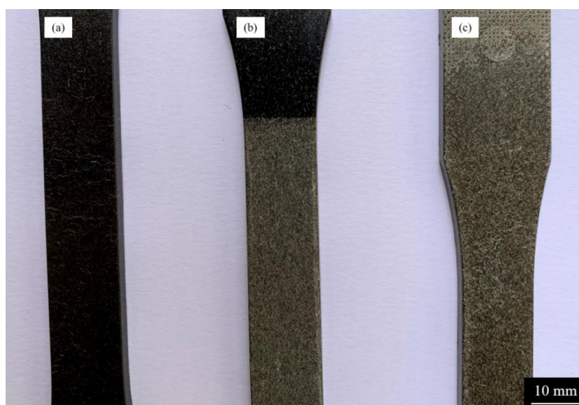
Figure 2. Visual non-destructive test of PPMCW sample (a) before, (b) after natural, and (c) accelerated aging.
