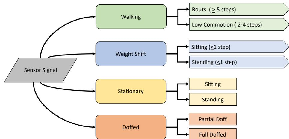
**Figure A3.** Diagram illustrating the prosthesis use categories and sub-categories.
