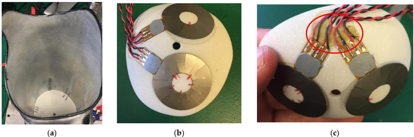
**Figure 3.** Insert assembly and placement into a socket. (a) Marks are inked on the insert and socket during a dry run assembly to facilitate proper alignment. (b) Antennae are affixed to the insert using hot melt, and annular-shaped Ferrite disks are affixed using double-sided tape. (c) Leadwires are covered with hot melt.
