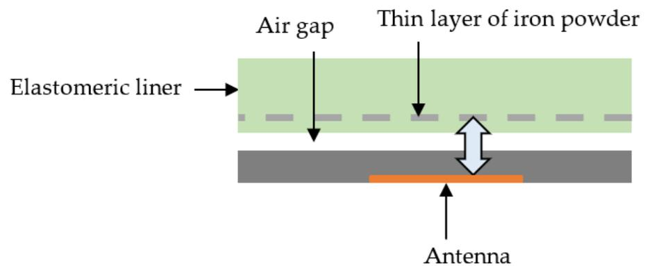
**Figure A1.** Sensor in a socket. The antenna is on the bottom side of the insert. The system measures the distance between the antenna and the iron powder within the liner (light blue double arrow). The system is calibrated to record the distance between the inside of the insert and the outside of the liner.
