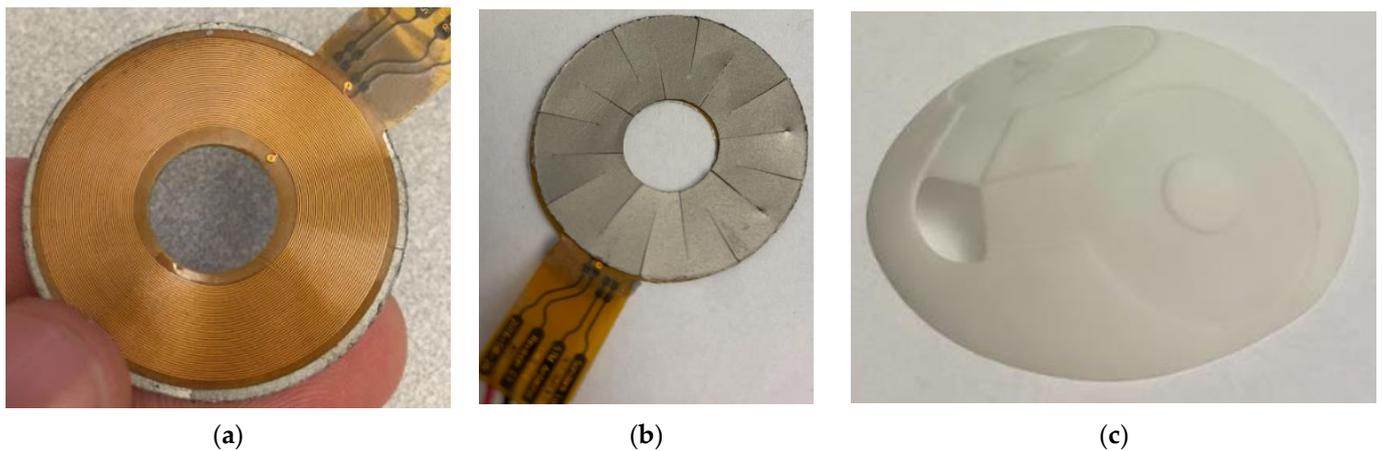
**Figure 2.** Sensor antenna. (a) Custom antenna with the center removed to improve flexibility. (b) A thin piece of ferrite is adhered to the external surface, and radial slits are made to improve flexibility. (c) Bottom view of a fabricated insert ready for antenna and leadwire attachment.
