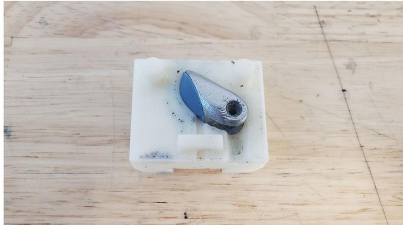
**Figure 5.** Overmolding achieved on additive manufactured component moulded using a silicon elastomer in a chamber produced by additive manufacturing.
