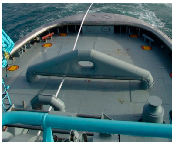
Figure 13. Wide staple of Escort Voith Water Tractor Tug “Tenax” with water spray cooling for escort towing with a high modulus polyethylene (HMPE) towline. The contact surfaces of both the staple and all around the cap rail are made of a highly polished stainless steel. Photo: Authors.
