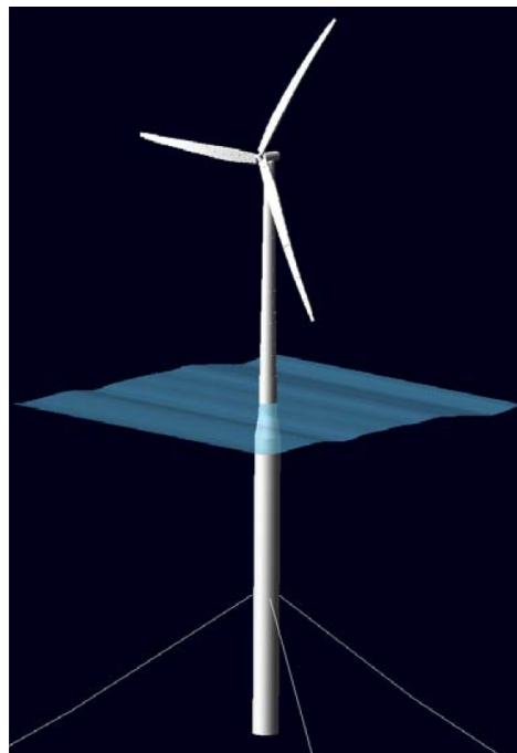
Figure 6. The OC3 floating spar-buoy wind turbine system [63].
