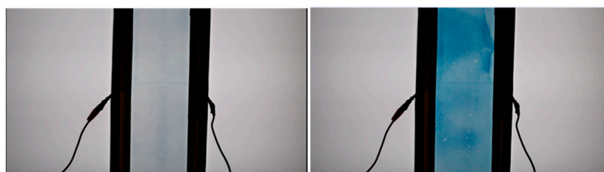
Figure 5. Clear and dark states of a 360\text{ cm}^2 active area PEDOT-PSS/ \text{V}_2\text{O}_5 assembled device, under D65 standard illumination conditions, cycled between +0.5 V to −4 V.
