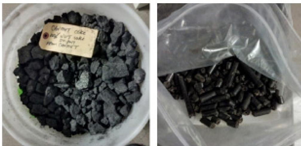
**Figure 1.** Appearance of nut coke (left) and torrefied wood pellets (right).
