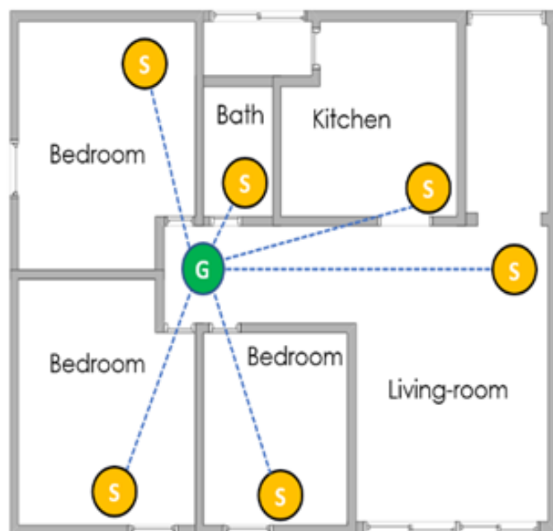
Figure 6. WSN topology of the pilot apartments in Spain.
