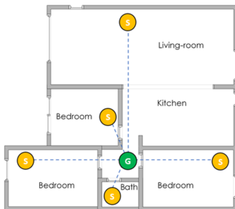
Figure 7. WSN topology of the pilot apartments in Greece.
