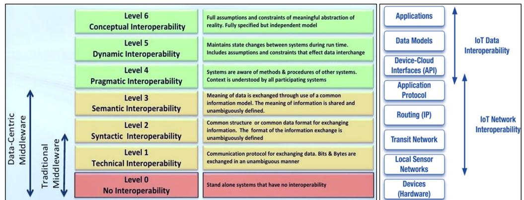
Figure 2. The interfacing levels of the interoperability model (adapted from [6]).
