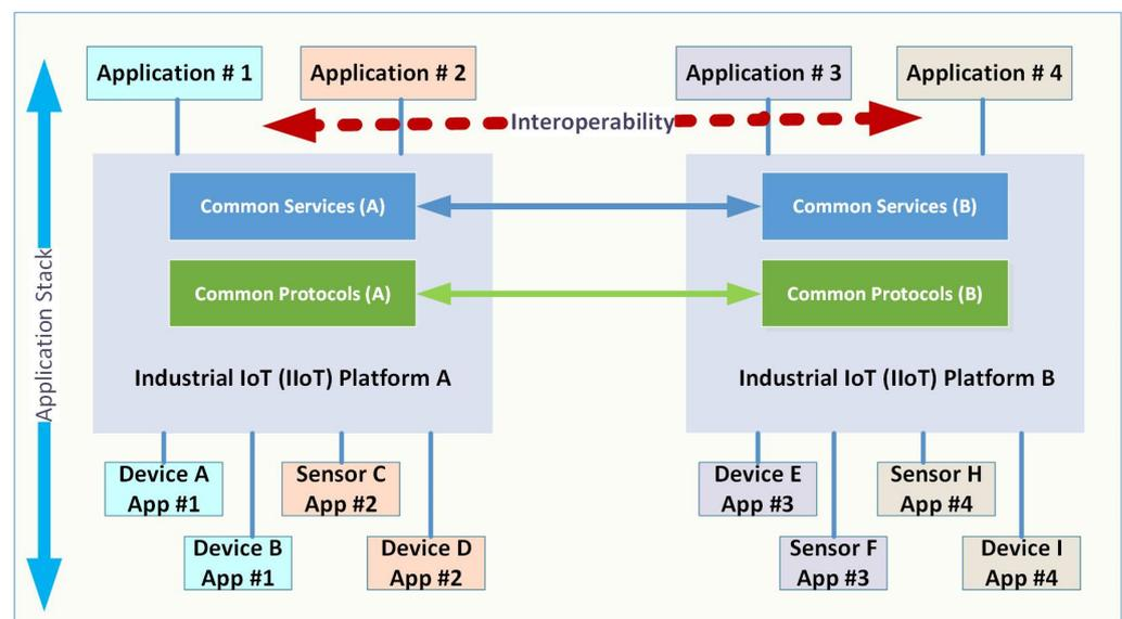
**Figure 3.** Schematic of semantic interoperability between different IoT platforms.
