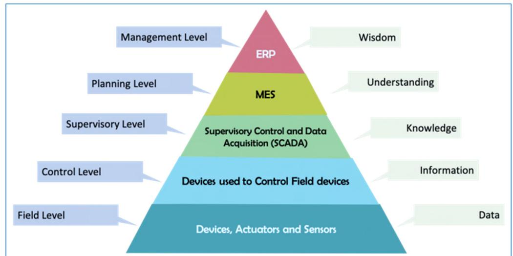
**Figure 1.** Automation pyramid (adapted from [1]).
