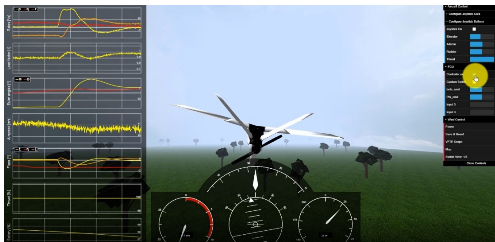
Figure 22. VFTE window view during the SIL co-simulation using the Simulink lateral observer/controller loop.
