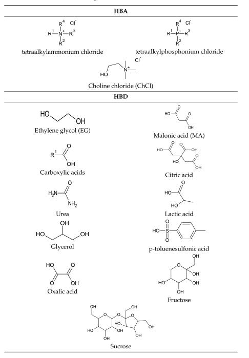
**Table 2.** Structure of the hydrogen bond donors (HBDs), and hydrogen bond acceptors (HBAs) for the synthesis of DESs used for metal leaching.
