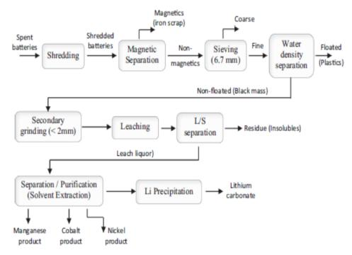
**Figure 1.** Hydrometallurgical flowsheet for the recovery of metals. Reproduced from [12] with permission from Elsevier.
