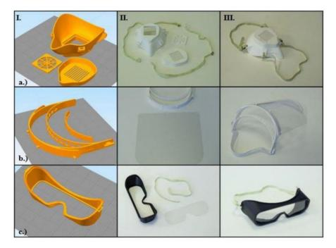
**Figure 1.** Overview of personal protective equipment (PPE) manufacturing process using 3D printing. With Column I—demonstrating CAD assembly, II—3D printed parts, III—the assembled models. The rows show (**a**) a respirator face mask; (**b**) a face shield; (**c**) a pair of safety googles. This image is reprinted under a Creative Commons Attribution 4.0 International License and it is taken from [18].
