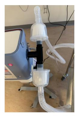
**Figure 3.** A 3D printed T-Piece Ventilator Splitter connected to a ventilator. This image is reprinted under a Creative Commons Attribution 4.0 International License and it is from [50].
