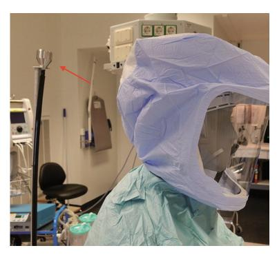
**Figure 5.** Stryker Flyte modified ventilated helmet using 3D printing to facilitate powered air filter units and improve safety. This image is reprinted under a Creative Commons Attribution 4.0 International License and it is taken from [80].
