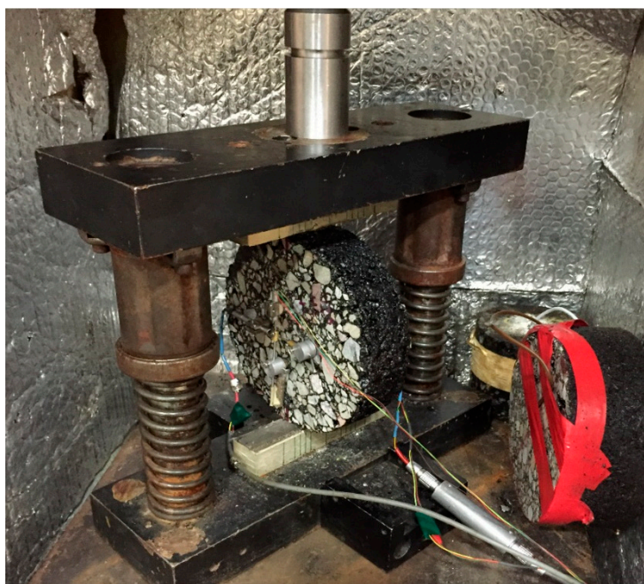
Figure 5. Instrumentation of the specimens for creep compliance testing.
