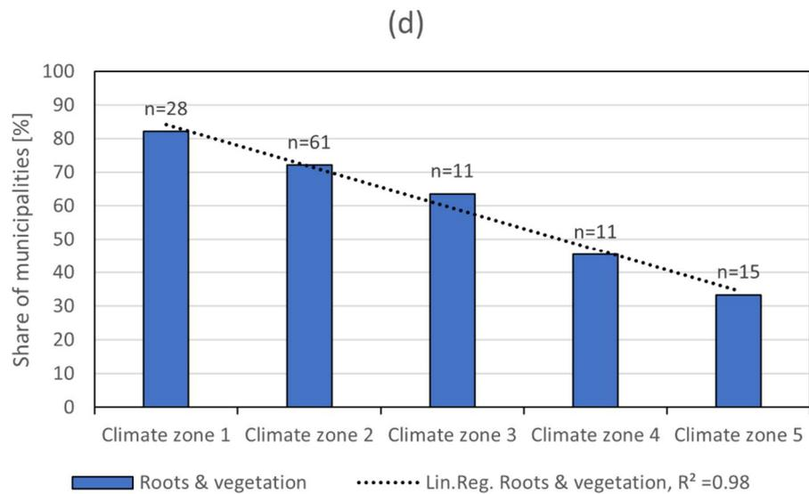
**Figure 8.** Problematic frequency of distress causes on the municipal cycle path networks with respect to climate zones for (a) frost heave, (b) freeze and thaw cycles, (c) poor material/poor execution, and (d) roots and vegetation.
