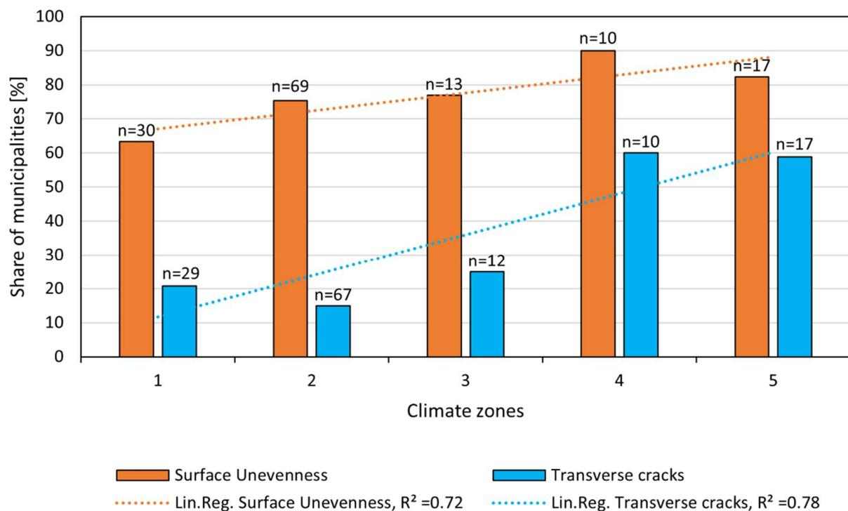
**Figure 4.** The correlation of the stated problematic frequency of surface unevenness and transverse cracks on municipal cycle paths with the climate zones in TRVK Väg.
