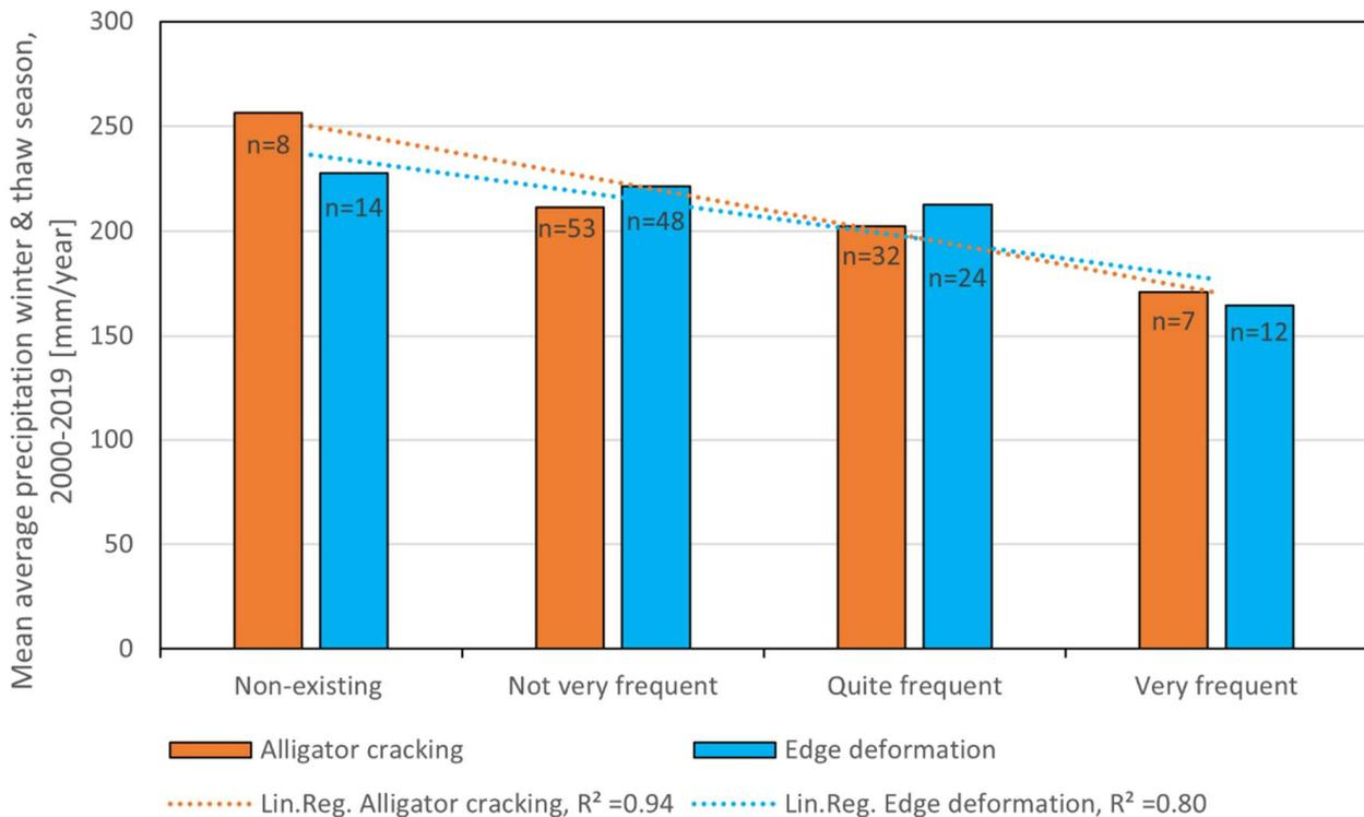
**Figure 5.** The correlation of the stated frequency of alligator cracking and edge deformation on municipal cycle paths and the mean average precipitation for winter and thaw seasons 2000–2019.
