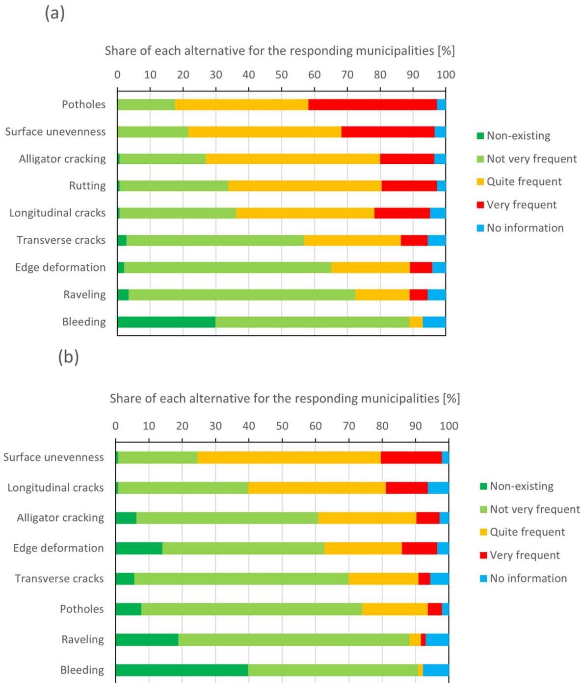
**Figure 3.** The stated frequency of distress by type on the municipal (a) streets and (b) cycle path networks, respectively. The response rate varies for the different distress modes and is marginally higher for streets (n = 144–148) than for cycle paths (n = 141–143).
