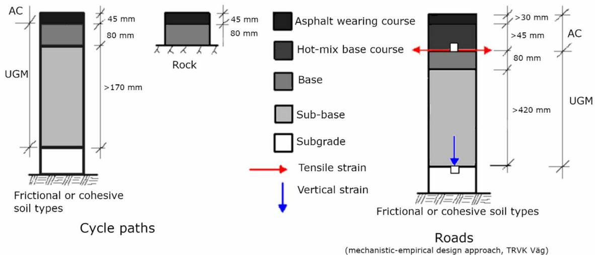
**Figure 1.** The structural design, with stipulated layer thicknesses of cycle paths and roads in the Swedish road- and street-design manual, *TRVK Väg*. The red arrows represent the design criteria of the tensile strain at the bottom of the AC layer, and the blue arrow represents the design criteria of the vertical strain on top of the subgrade.
