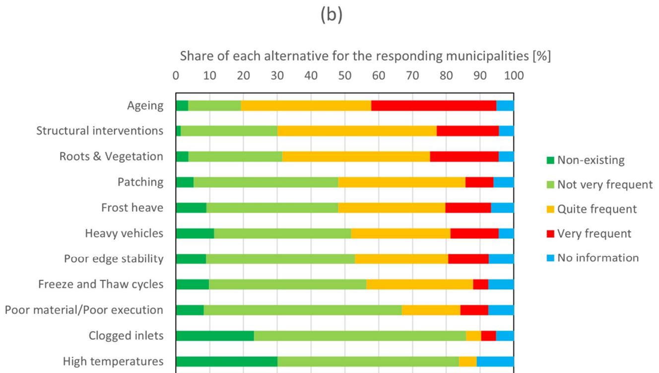
**Figure 7.** Stated causes of distress on the municipal (a) street- and (b) cycle-path network. The response rate varies for the different distress causes and is marginally higher for streets ( $n = 136\text{--}140$ ) than for cycle paths ( $n = 133\text{--}136$ ).
