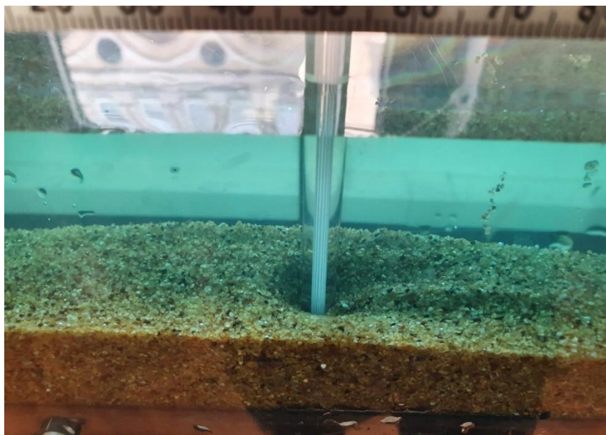
Figure 15. Example of a scour hole formation for stone gabion (thickness 8 mm) at a sediment depth of 40 mm.
