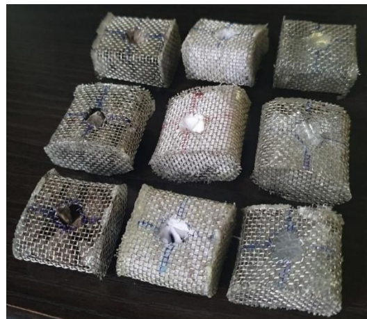
Figure 7. Image of gabion boxes with various dimensions and fill increasing in height from bottom to top: 8 mm, 12 mm and 16 mm (from left to right: stone, clothing, plastic).
