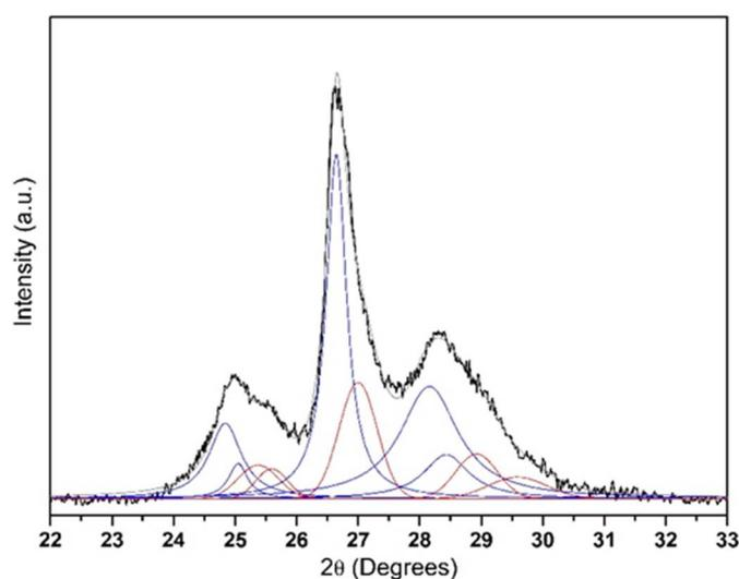
**Figure S1.** Representative example of the peak broadening deconvolution analysis of the XRD profiles (AgCdS-T sample).
