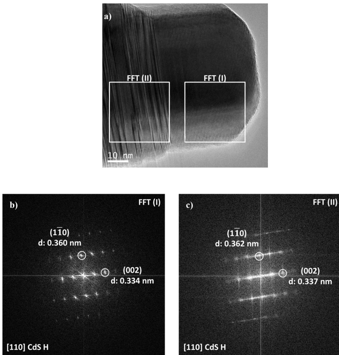
**Figure S7.** HR-TEM images of the FFT analysis for the determination of the crystalline planes of the (a) AgCdS-S for the region FFT I (b) and FFT II (c).
