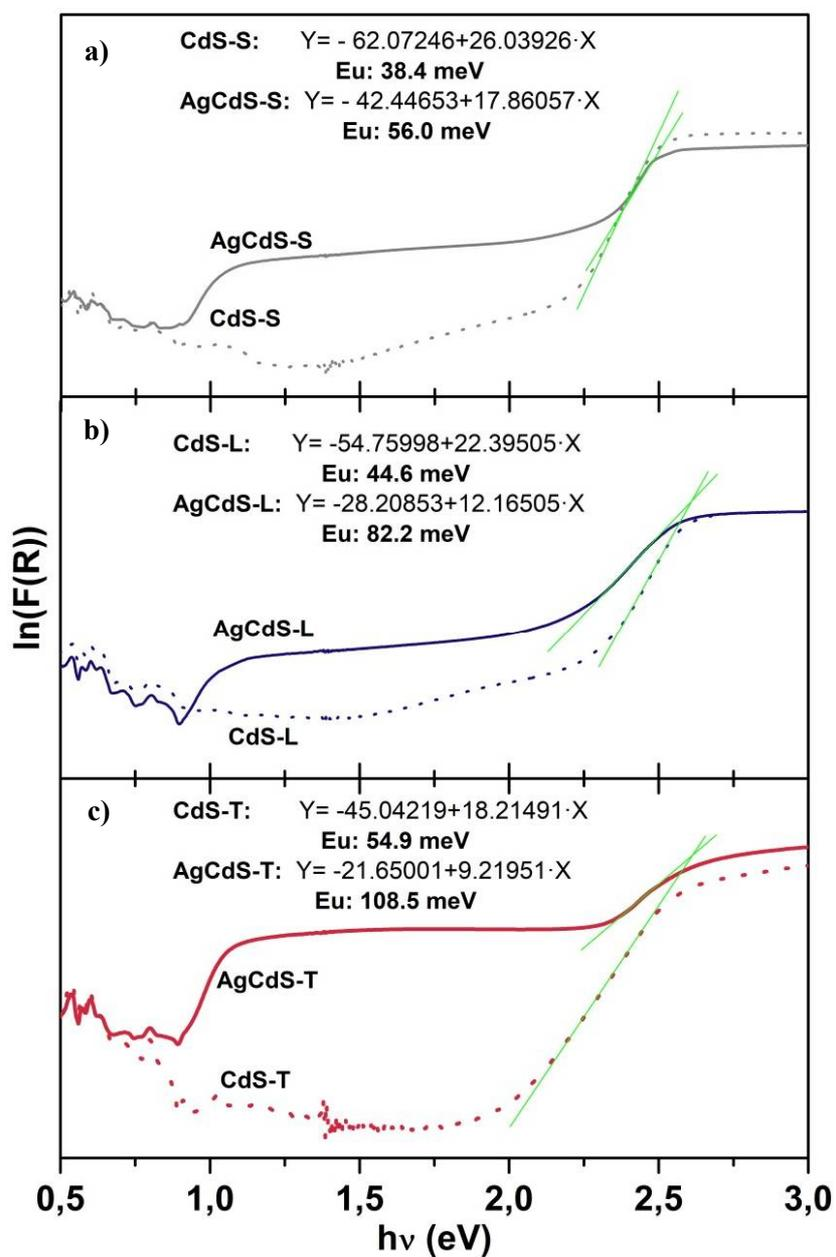
**Figure S8.** Urbach tails linear fit of CdS-X and AgCdS-X photocatalysts prepared with different sulphur sources: a) Elemental sulfur b) L-cysteine and d) thiourea.
