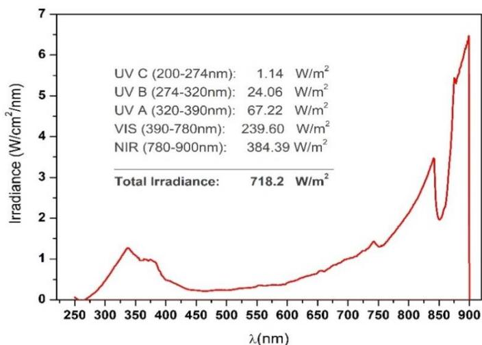
**Figure S3.** Irradiance spectra of the Xe arc lamp (150W, ozone Free, LOT Oriel GmbH & CO KG) measured with spectroradiometer (ILT550 LOT Oriel GmbH & Co. KG) at a focal distance equal to 26.5 cm.
