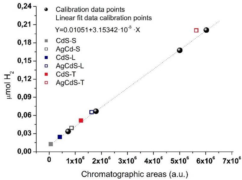
**Figure S5.** H<sub>2</sub> calibration curve for the quantification of the hydrogen produced from the chromatographic areas and experimental fitting of the results obtained in the CdS-X and AgCdS-X samples.
