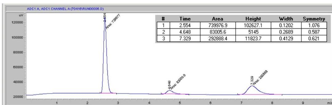
**Figure S4.** Representative chromatogram (AgCdS-S sample) obtained in the GC Varian STAR CX3400 to quantify the produced H<sub>2</sub> (peak at retention time 2.55 min).
