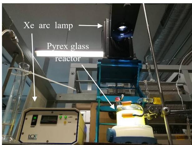
**Figure S2.** Experimental setup used for the photocatalytic activity measurements.
