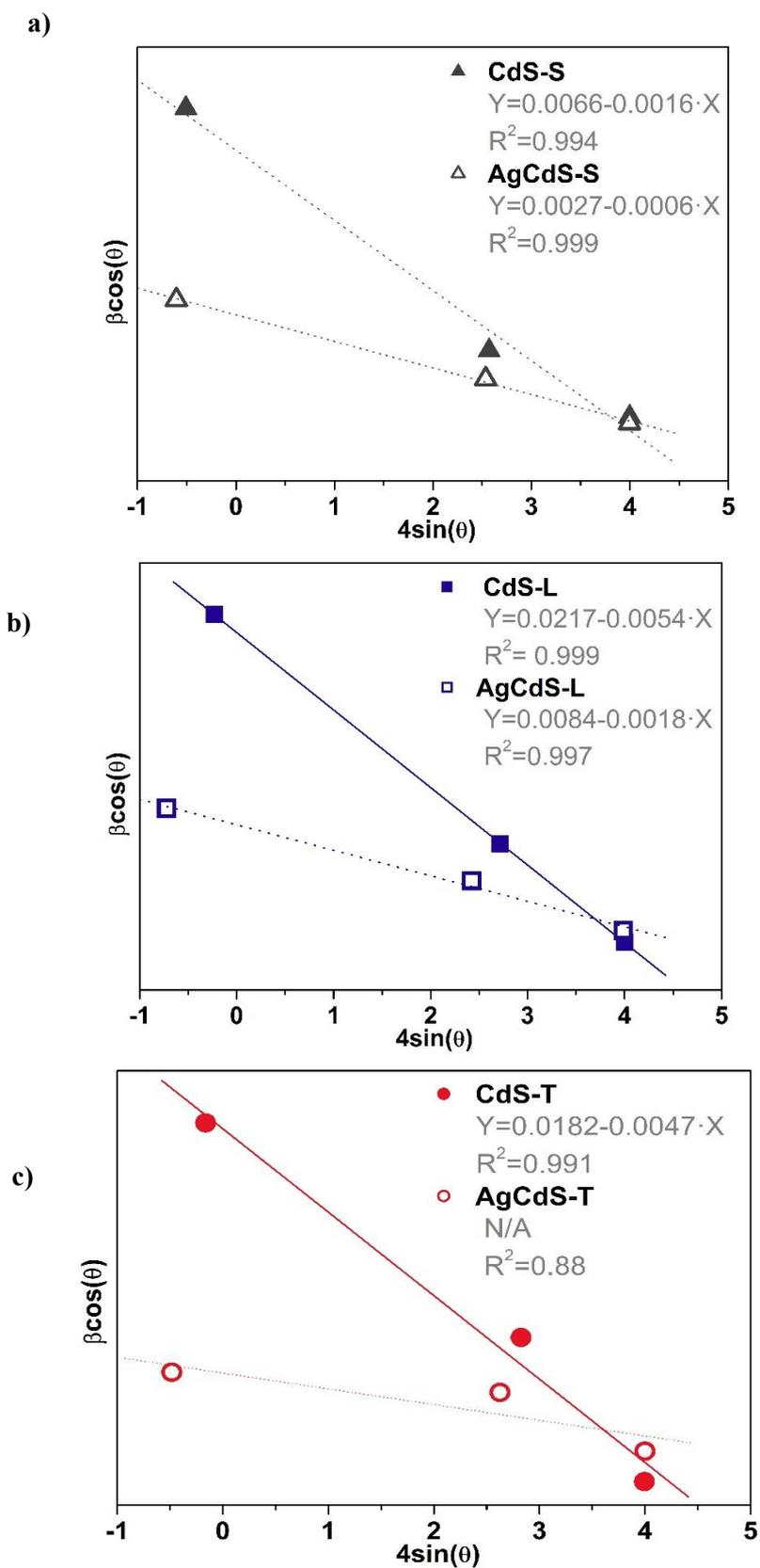
**Figure S6.** Williamson-Hall plot linear fit for the CdS-X and AgCdS-X photocatalysts prepared with different sulphur source: a) Elemental sulfur, b) L-cysteine and c) Thiourea.
