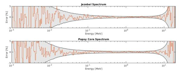
Figure 3. Error in flux spectrum for the fast benchmark cases. Grey region represents the extent of two standard deviations.
