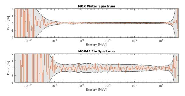
Figure 4. Error in flux spectrum for the MOX thermal benchmark case. Grey region represents the extent of two standard deviations.
