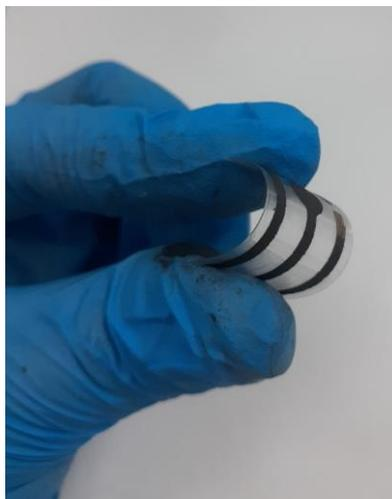
**Figure 3.** Demonstration of ink flexibility on the printed electrode.
