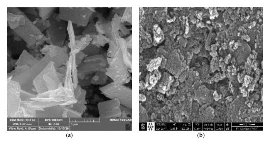
**Figure 2.** The FE-SEM images of  $Bi_2O_3$  nanoparticles. (a) Method A (1  $\mu$ m) (b) Method B (500 nm).
