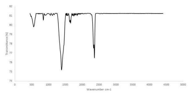
Figure 1. The FTIR spectra of Bi<sub>2</sub>O<sub>3</sub> nanoparticles.
